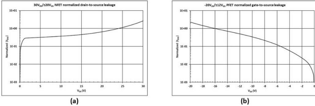
**Figure 5. I<sub>DSS</sub> Vs. v<sub>DS</sub> With No ESD Protection: 30-v NFET (a); and –20-v PFET (b)**
