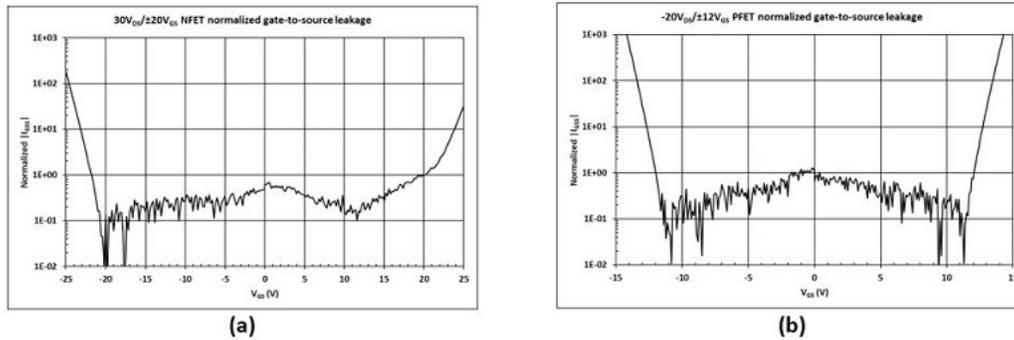
Figure 2.  $I_{GSS}$  Vs.  $v_{GS}$  With No ESD Protection: 30-v NFET (a); and -20-v PFET (b)
