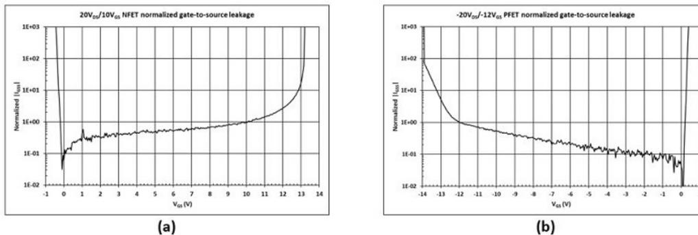
Figure 3.  $I_{GSS}$  vs.  $V_{GS}$  with single-ended ESD protection: 20-V NFET (a); and -20-V PFET (b)
