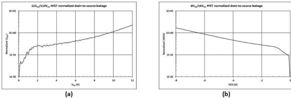
**Figure 7. I<sub>DSS</sub> Vs. v<sub>DS</sub> With Back-to-back ESD Protection: 12-v NFET (a); and –20-v PFET (b)**
