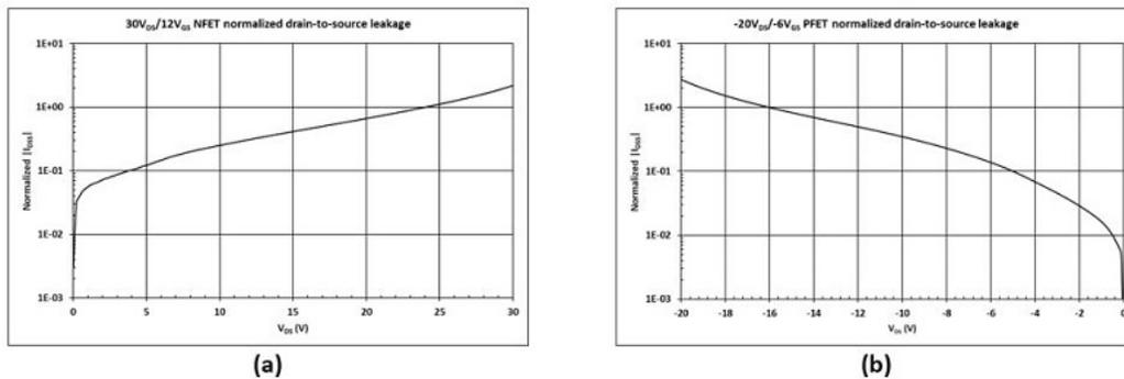
**Figure 6. I<sub>DSS</sub> Vs. v<sub>DS</sub> With Single-ended ESD Protection: 20-v NFET (a); and –20-v PFET (b)**
