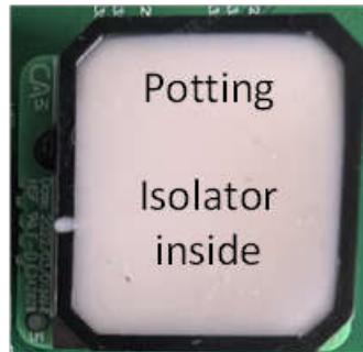
Figure 5-3. Potting Method to Achieve Solid Insulation
