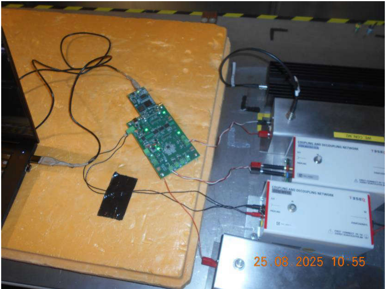
Figure 3-15. Laboratory Setup for CI Test
