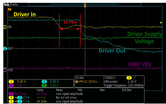
Figure 8-5. Turn-Off Propagation Delay Waveform
