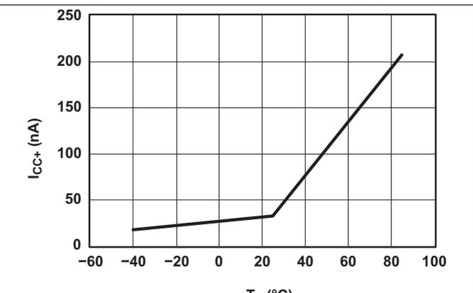
Figure 12. Power-Supply Current vs Temperature ( $V_+ = 5\text{ V}$ )
