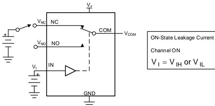
Figure 15. ON-State Leakage Current ( $I_{COM(ON)}$ ,  $I_{NC(ON)}$ ,  $I_{NO(ON)}$ )
