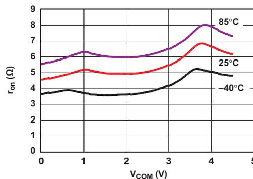
Figure 26.  $r_{on}$  vs  $V_{COM}$ ,  $V_+ = 5$  V
