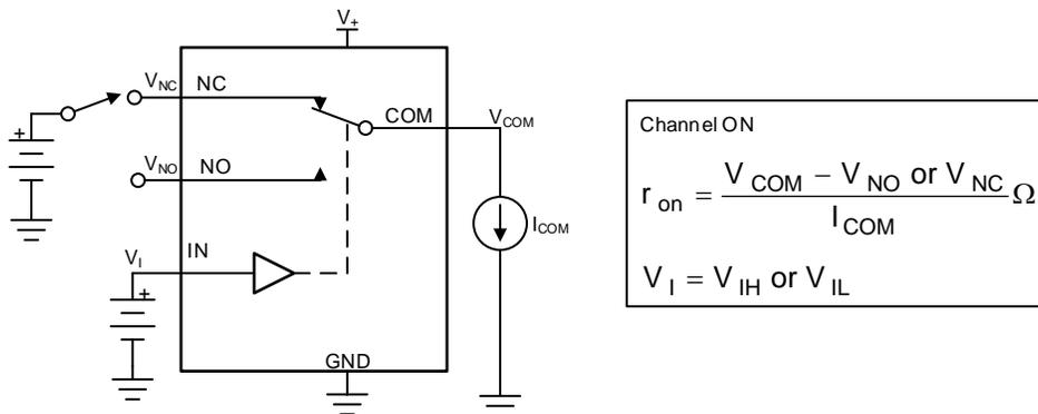
Figure 13. ON-State Resistance ( $r_{on}$ )
