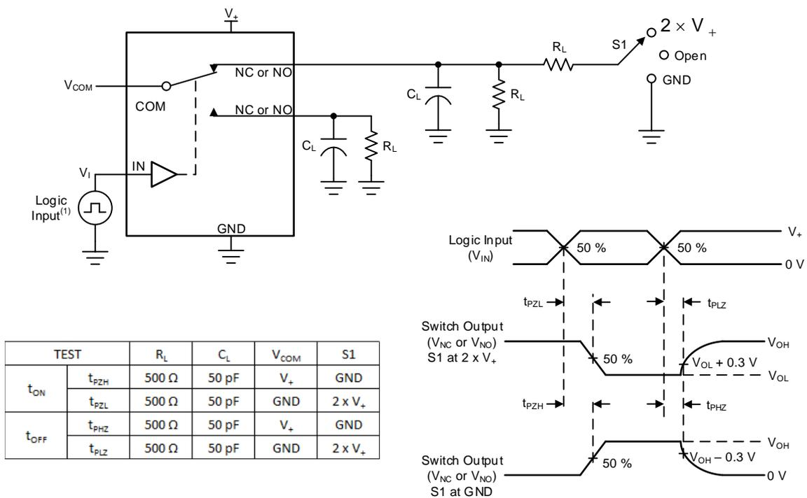
(1) All input pulses are supplied by generators having the following characteristics: PRR  $\leq$  10 MHz,  $Z_O = 50 \Omega$ ,  $t_r < 5$  ns,  $t_f < 5$  ns.
