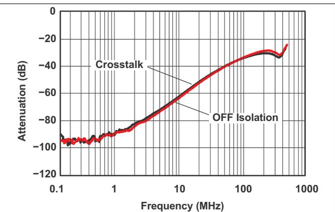
Figure 10. OFF Isolation and Crosstalk ( $V_+ = 3.3\text{ V}$ )
