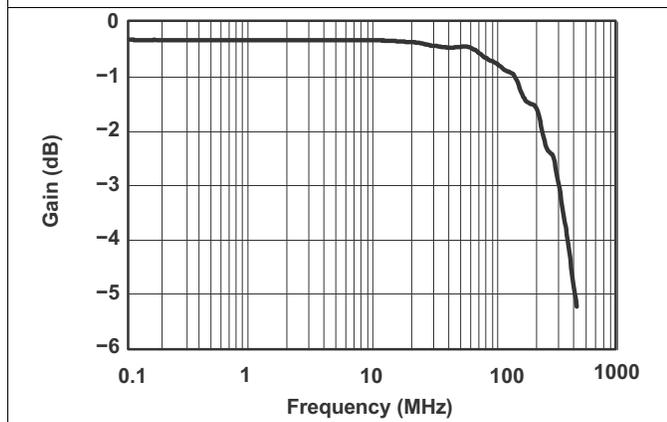
Figure 9. Bandwidth ( $V_+ = 3.3\text{ V}$ )
