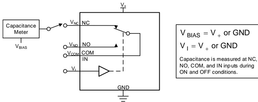
Figure 16. Capacitance ( $C_{IN}$ ,  $C_{COM(ON)}$ ,  $C_{NC(OFF)}$ ,  $C_{NO(OFF)}$ ,  $C_{NC(ON)}$ ,  $C_{NO(ON)}$ )
