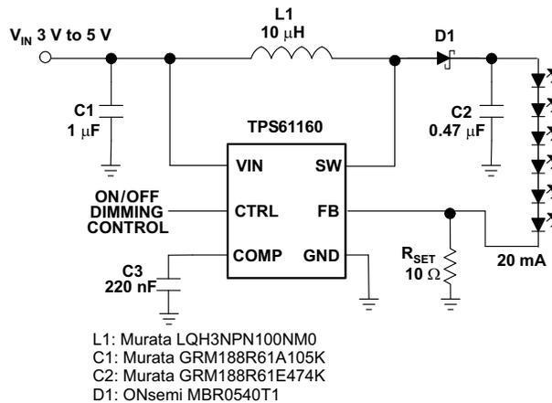
Figure 23. Li-Ion Driver for 6 White LEDs
