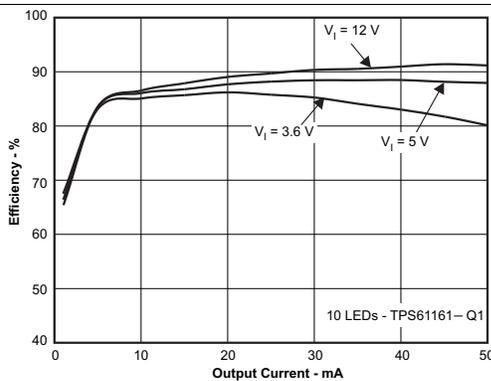
Figure 3. Efficiency vs Output Current
