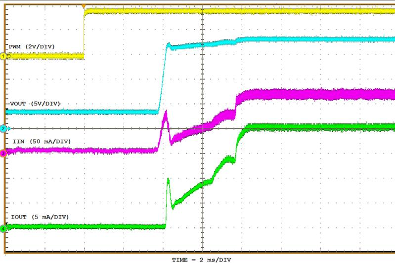
Figure 26. Start-Up with 6 Series LEDs ( $D_{PWM} = 100\%$ )
