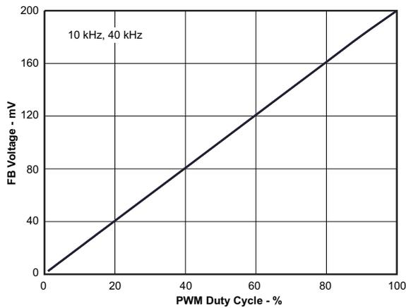
Figure 7. FB Voltage vs PWM Duty Cycle
