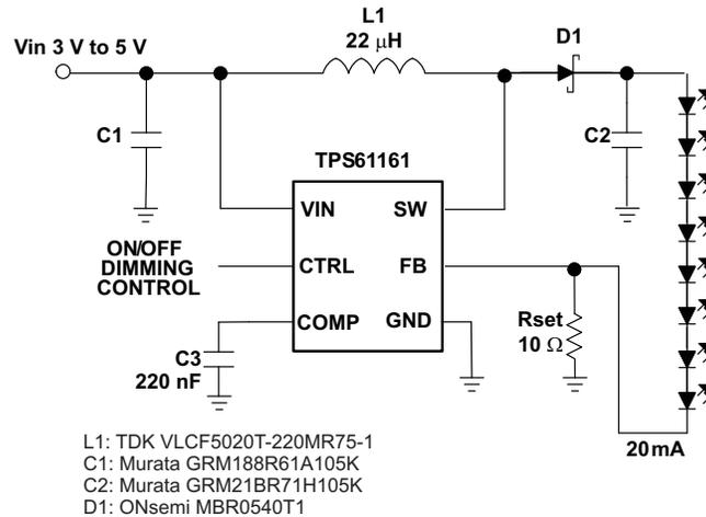
Figure 27. Li-Ion Driver for 8 White LEDs
