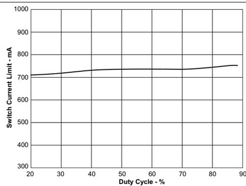
Figure 4. Switch Current Limit vs Duty Cycle
