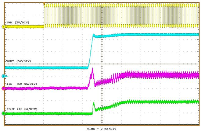
Figure 25. Start-Up with 6 Series LEDs ( $D_{PWM} = 50\%$ )
