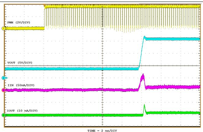
Figure 21. Start-Up with 6 Series LEDs (External PWM,  $D_{PWM} = 50\%$ )
