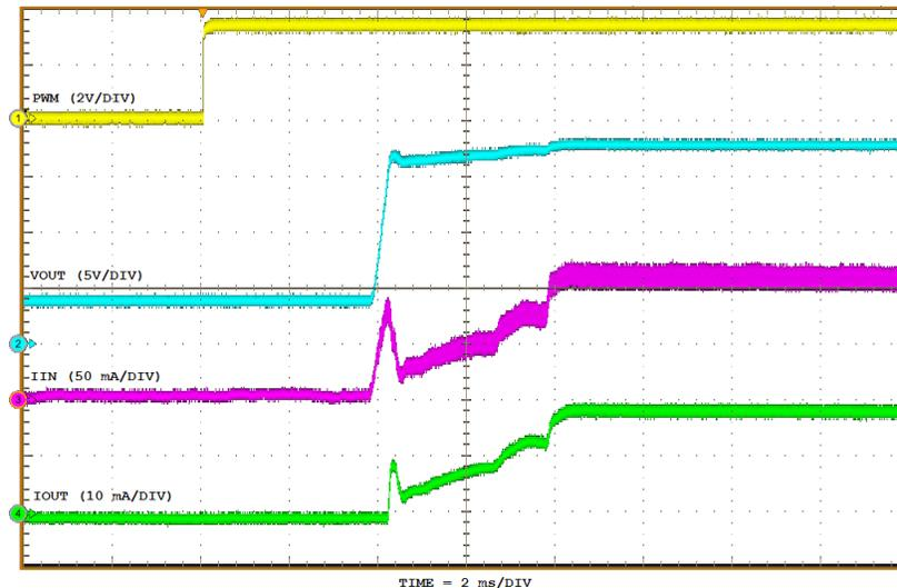
Figure 22. Start-Up with 6 Series LEDs (External PWM,  $D_{PWM} = 100\%$ )
