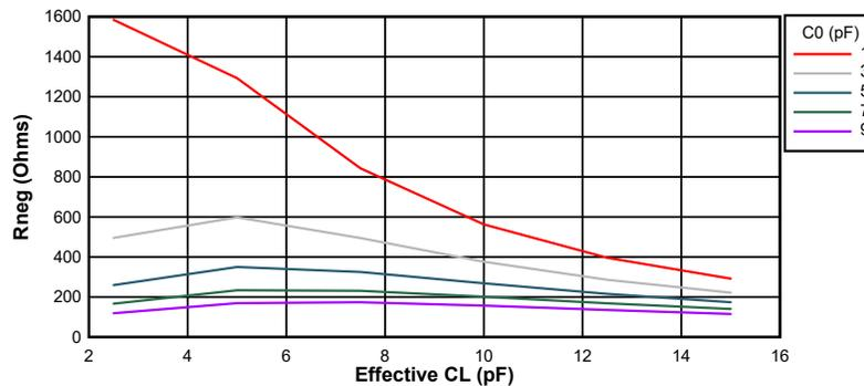
**Figure 6-23. Negative Resistance Variation at 20 MHz**
