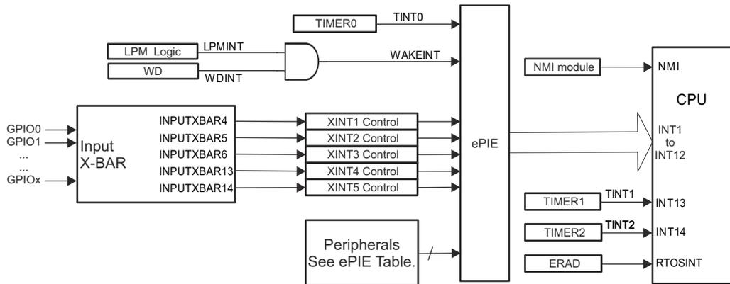
**Figure 6-33. Device Interrupt Architecture**
