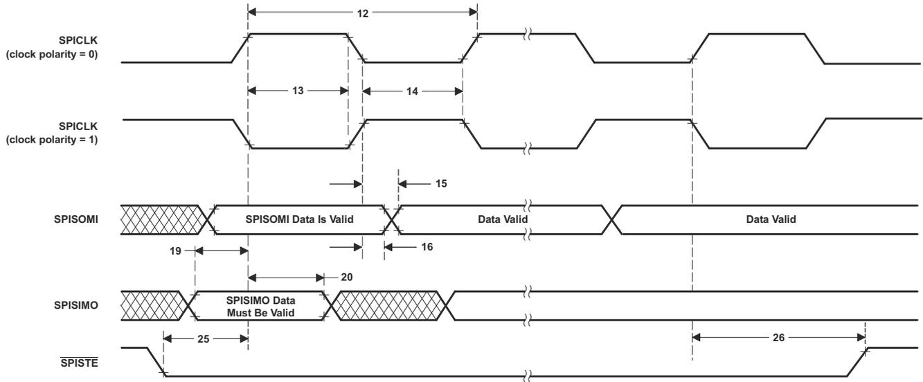
**Figure 6-87. SPI Slave Mode External Timing (Clock Phase = 1)**
