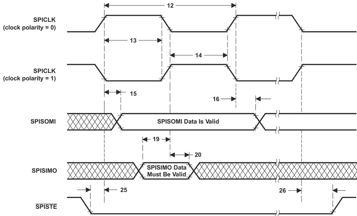
Figure 6-86. SPI Slave Mode External Timing (Clock Phase = 0)
