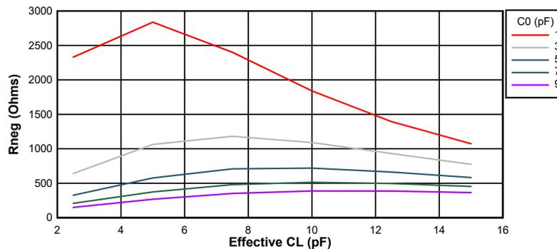
**Figure 6-22. Negative Resistance Variation at 10 MHz**
