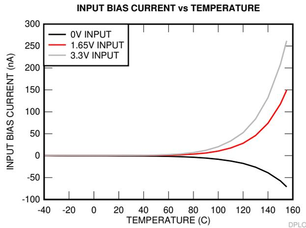
Figure 6-46. Input Bias Current Versus Temperature
