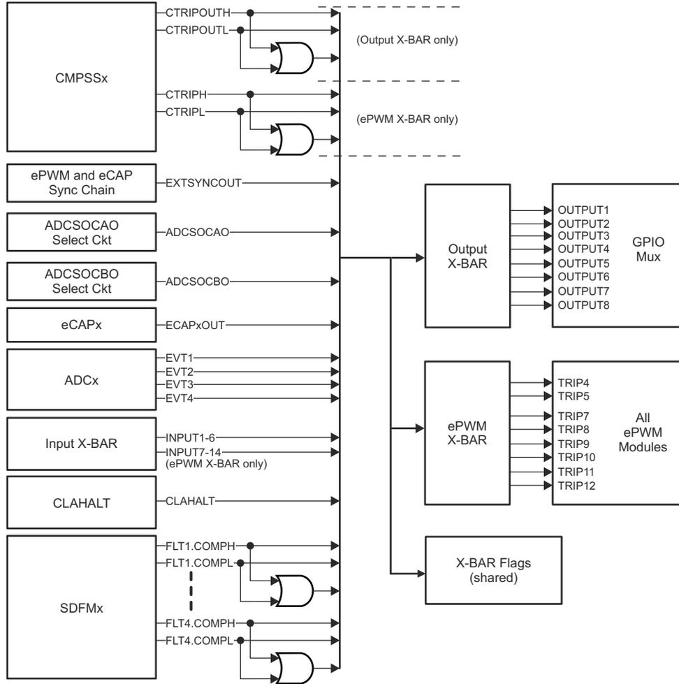
Figure 5-6. Output X-BAR and ePWM X-BAR Sources
