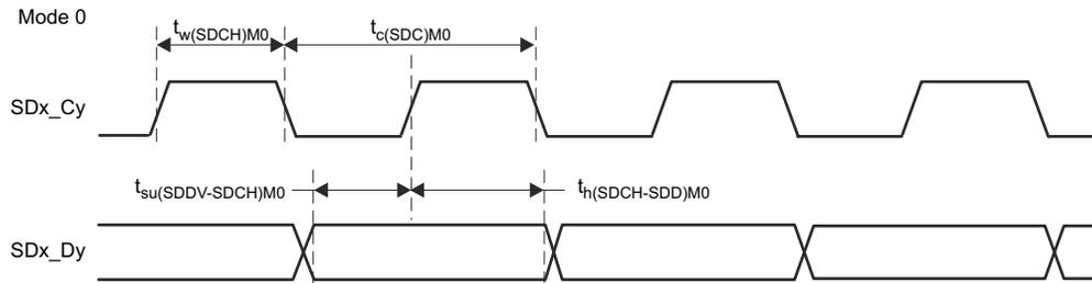
**Figure 6-74. SDFM Timing Diagram – Mode 0**
