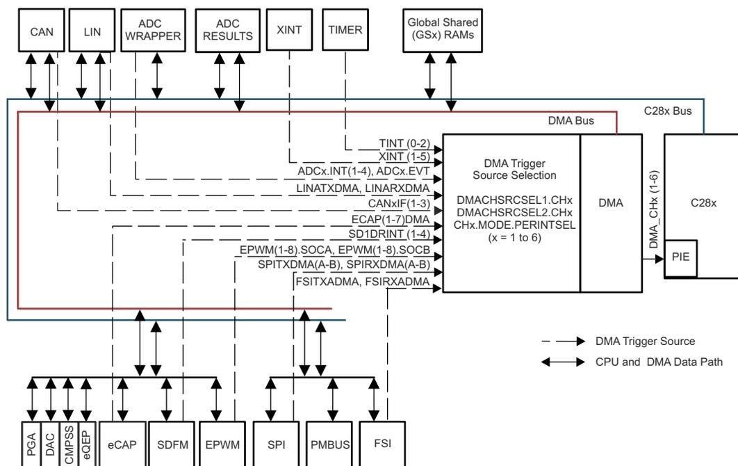
**Figure 7-3. DMA Block Diagram**
