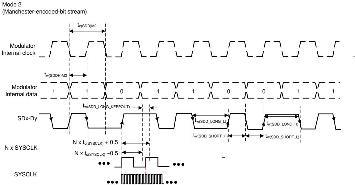
**Figure 6-76. SDFM Timing Diagram – Mode 2**
