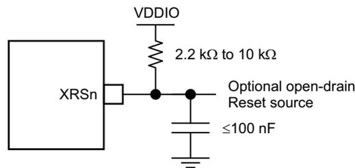
Figure 6-12. Reset Circuit
