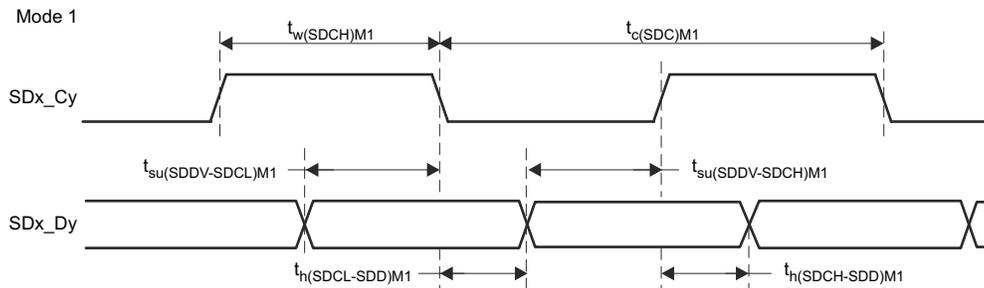
**Figure 6-75. SDFM Timing Diagram – Mode 1**
