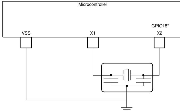
**Figure 6-19. External Resonator**
