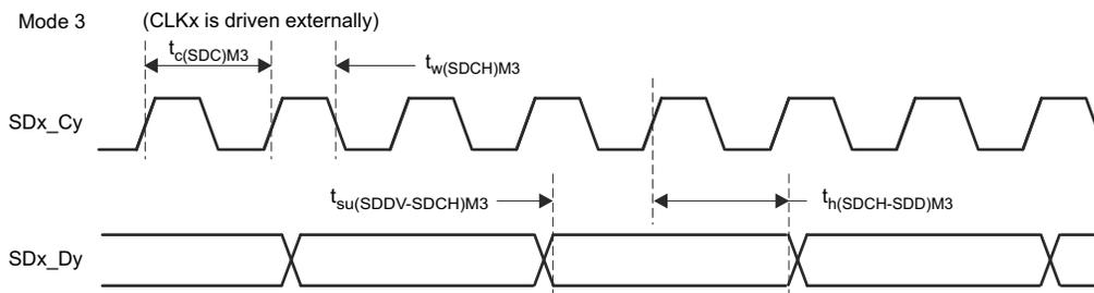
**Figure 6-77. SDFM Timing Diagram – Mode 3**
