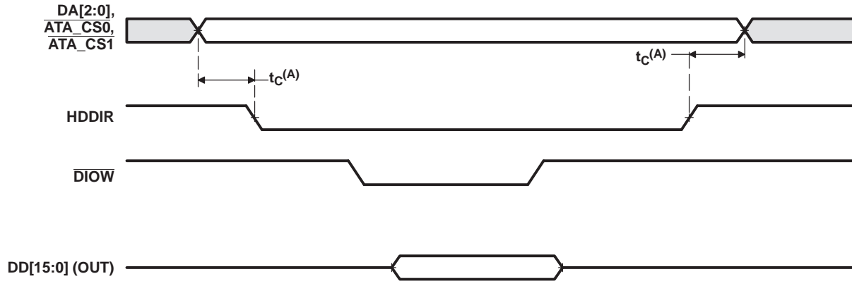
Figure 6-38. ATA/CF HDDIR Taskfile Write/Single PIO Write Timing
