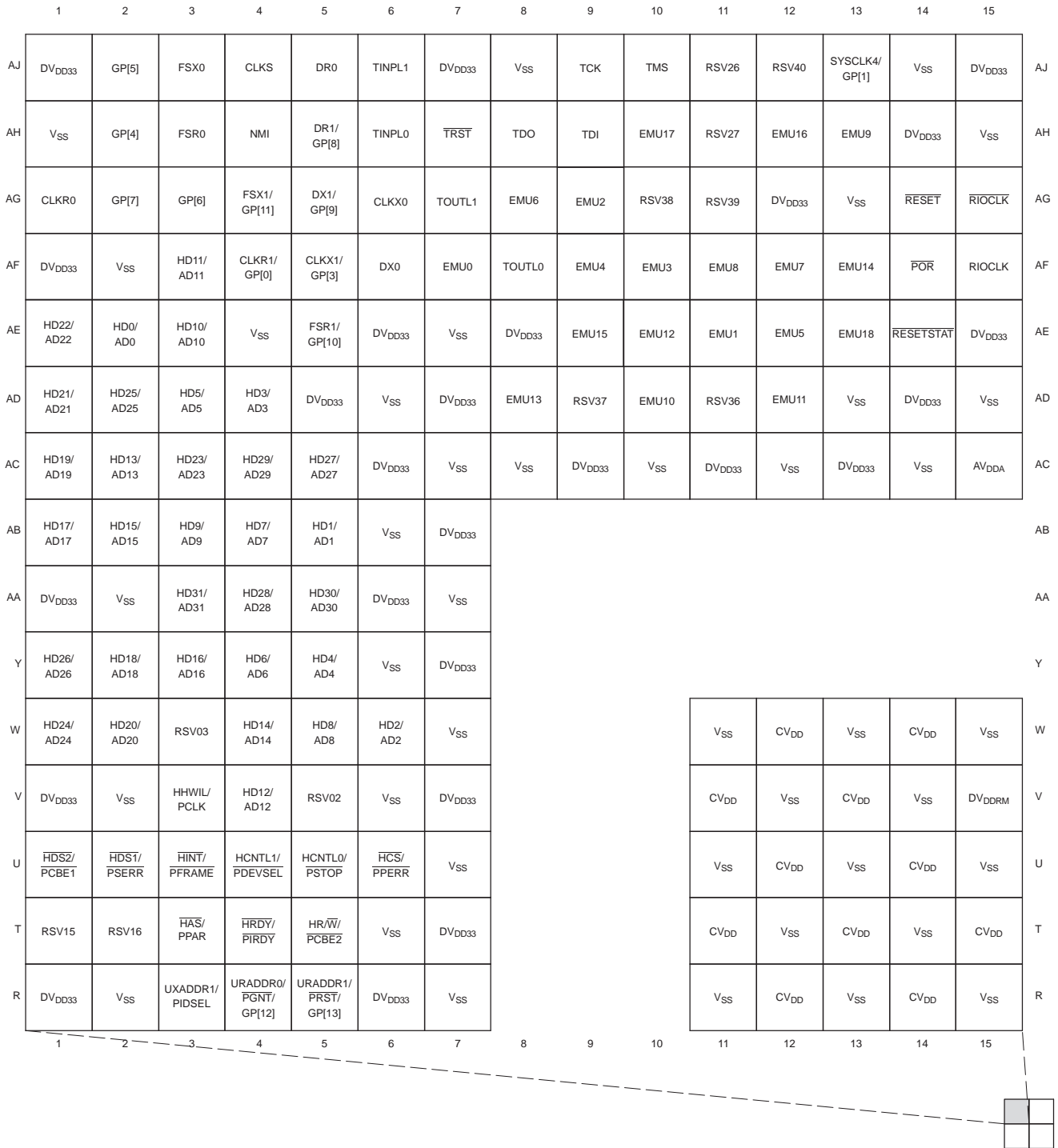
Figure 2-2. C6455 Pin Map (Bottom View) [Quadrant A]
