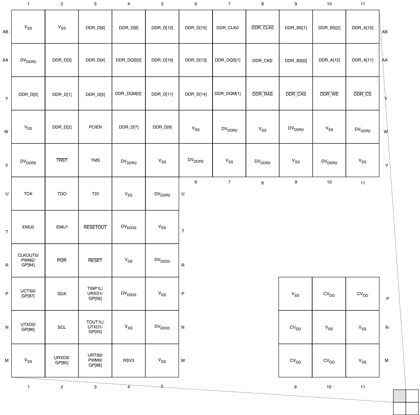
Figure 2-10. ZDU Pin Map [Quadrant A]
