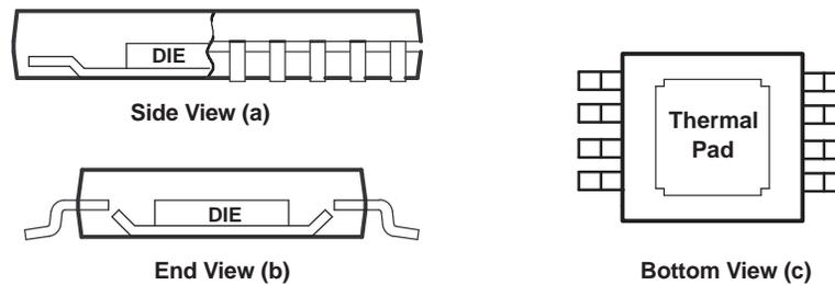
The thermal pad is electrically isolated from all terminals in the package.
