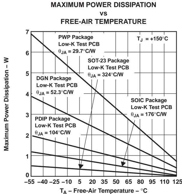
Results are obtained with no air flow and using JEDEC Standard Low-K test PCB.
