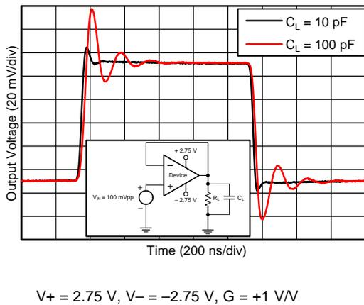
Figure 29. Small-Signal Step Response
