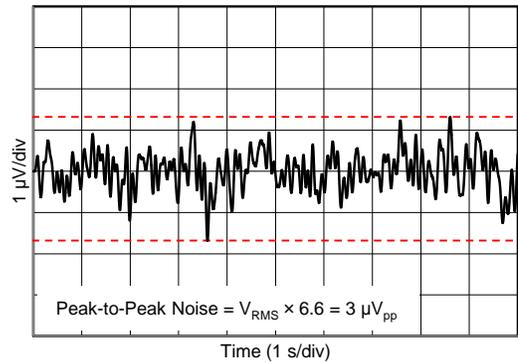
Figure 16. 0.1-Hz to 10-Hz Input Voltage Noise
