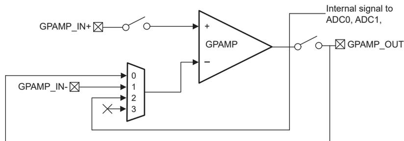
**Figure 8-2. Analog Connections**
