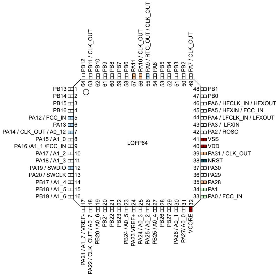
Figure 6-2. 64-Pin PM (LQFP) (Top View)
