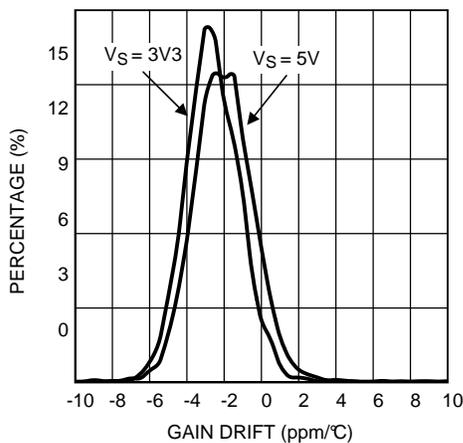
**Figure 39. Gain Drift Distribution, 5000 Parts LMP8602 and LMP8602-Q1**
