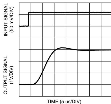
Figure 24. Settling Time (Rising Edge) at  $V_S = 5\text{ V}$
