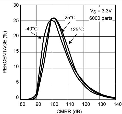
Figure 47. CMRR Distribution at  $V_S = 3.3\text{ V}$ , 6000 parts
