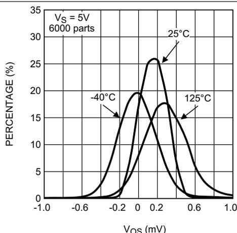
Figure 36.  $V_{\text{OS}}$  Distribution at  $V_S = 5\text{ V}$
