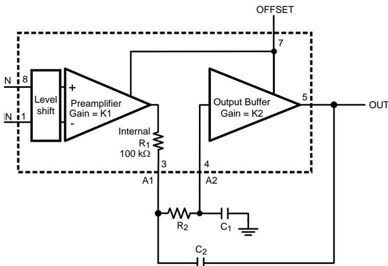
NOTE:  $K_1 = 10$ ;  $K_2 = 2$  for LMP8601, LMP8601-Q1; 5 for LMP8602, LMP8602-Q1; or 10 for LMP8603, LMP8603-Q1.
