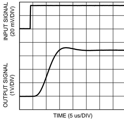
Figure 30. Settling Time (Rising Edge) at  $V_S = 5\text{ V}$
