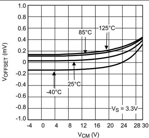
Figure 1.  $V_{\text{OS}}$  vs  $V_{\text{CM}}$  at  $V_S = 3.3\text{ V}$
