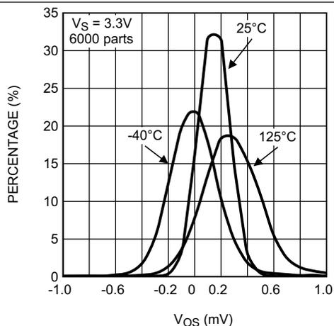
Figure 35.  $V_{\text{OS}}$  Distribution at  $V_S = 3.3\text{ V}$
