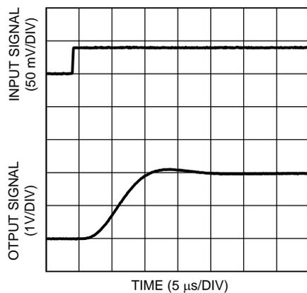
Figure 23. Settling Time (Rising Edge) at  $V_S = 3.3\text{ V}$
