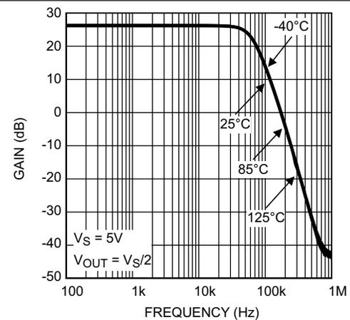
Figure 10. Gain vs Frequency at  $V_S = 5\text{ V}$
