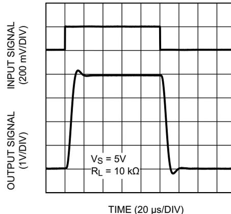
Figure 14. Step Response at  $V_S = 5\text{ V}$
