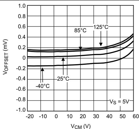
Figure 2.  $V_{\text{OS}}$  vs  $V_{\text{CM}}$  at  $V_S = 5\text{ V}$
