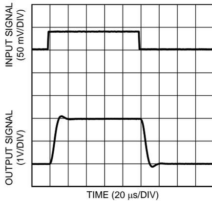
Figure 19. Step Response at  $V_S = 3.3\text{ V}$ ,  $R_L = 10\text{ k}\Omega$
