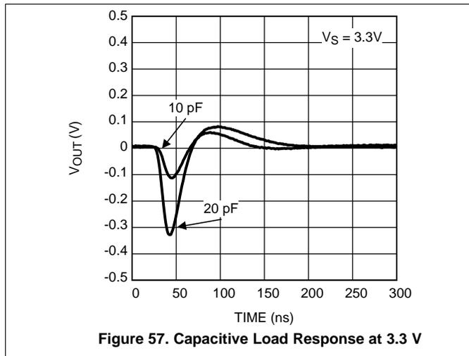
Figure 57. Capacitive Load Response at 3.3 V
