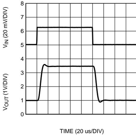
Figure 25. Step Response at  $V_S = 3.3\text{ V}$ ,  $R_L = 10\text{ k}\Omega$
