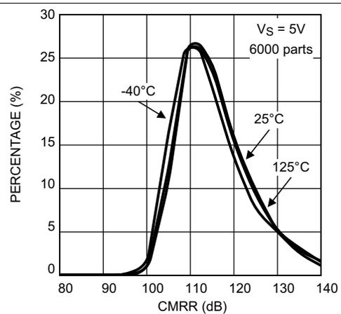
Figure 48. CMRR Distribution at  $V_S = 5\text{ V}$ , 6000 parts
