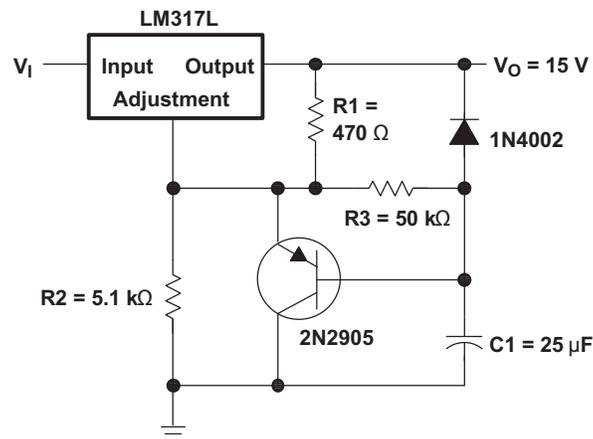
Figure 7-7. Slow-Turn On of the 15V Regulator Circuit
