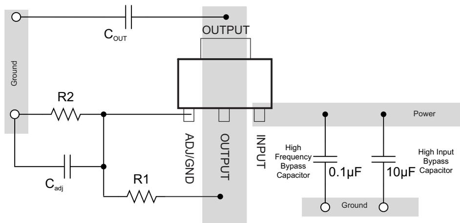
Figure 7-11. Layout Diagram
