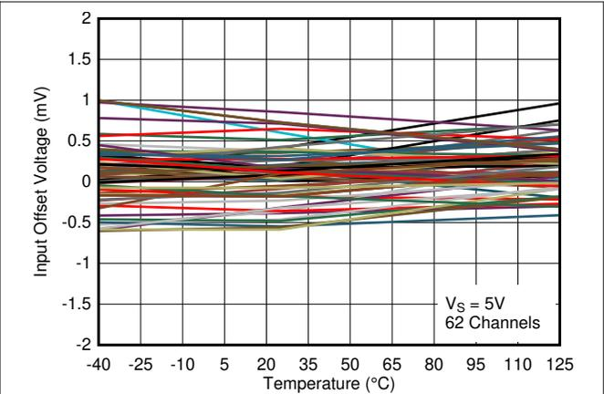
Figure 5-8. Input Offset Voltage vs. Temperature at 5V
