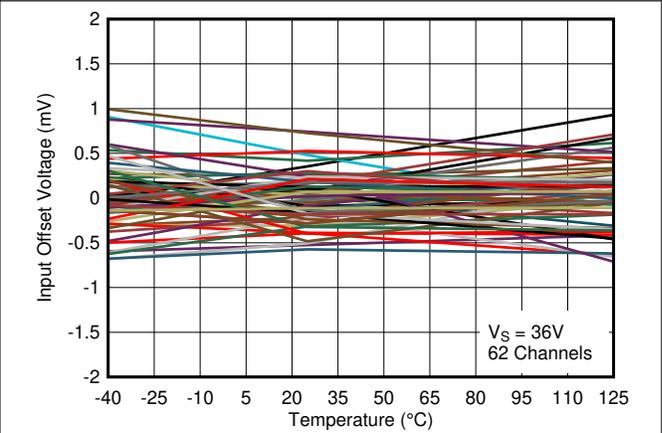
Figure 5-10. Input Offset Voltage vs. Temperature at 36V
