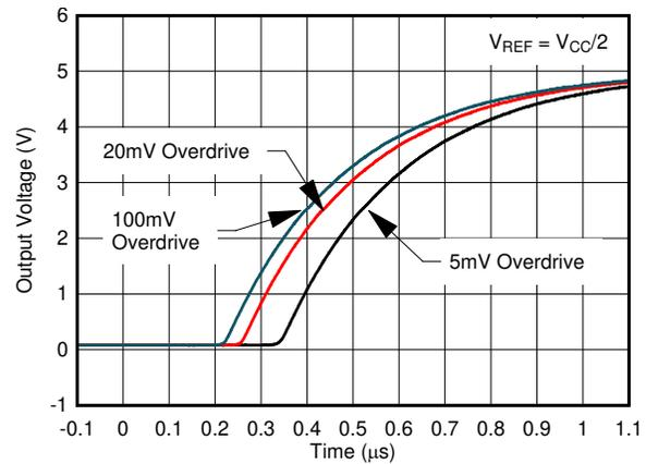
**Figure 5-32. Response Time for Various Overdrives, Low-to-High Transition**
