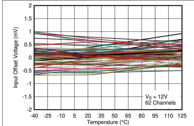
Figure 5-9. Input Offset Voltage vs. Temperature at 12V
