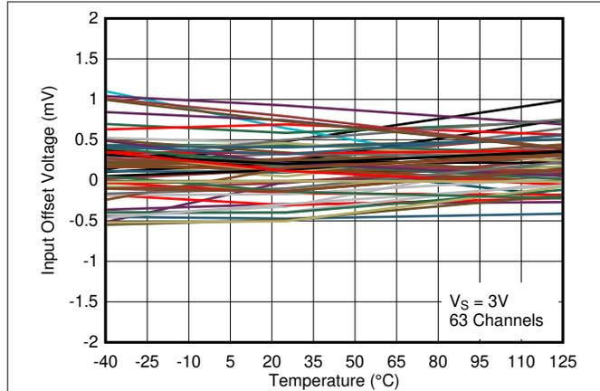
Figure 5-7. Input Offset Voltage vs. Temperature at 3V
