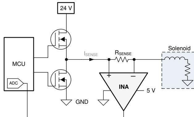
**Figure 7-2. Current Sensing in a Solenoid Application**
