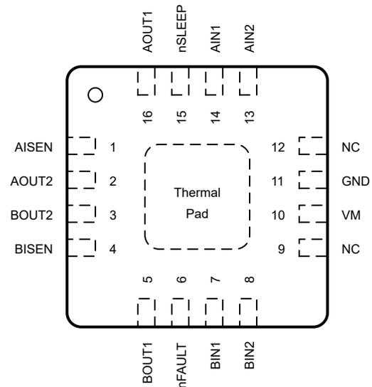
**Figure 5-2. RTE Package 16-Pin WQFN Top View**
