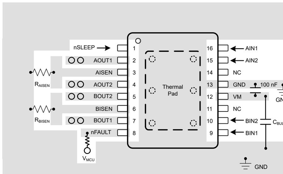
**Figure 9-24. Recommended Layout Example for PWP (HTSSOP) Package**
