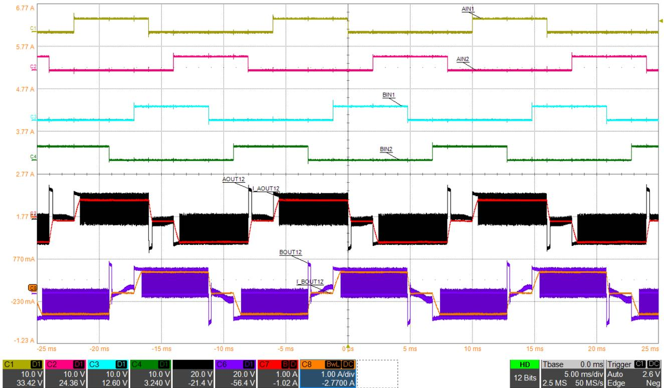
Figure 9-6. Stepper Motor Half-Step Operation With Fast Decay
