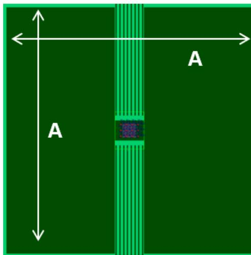
Figure 9-11. HTSSOP PCB model top layer
