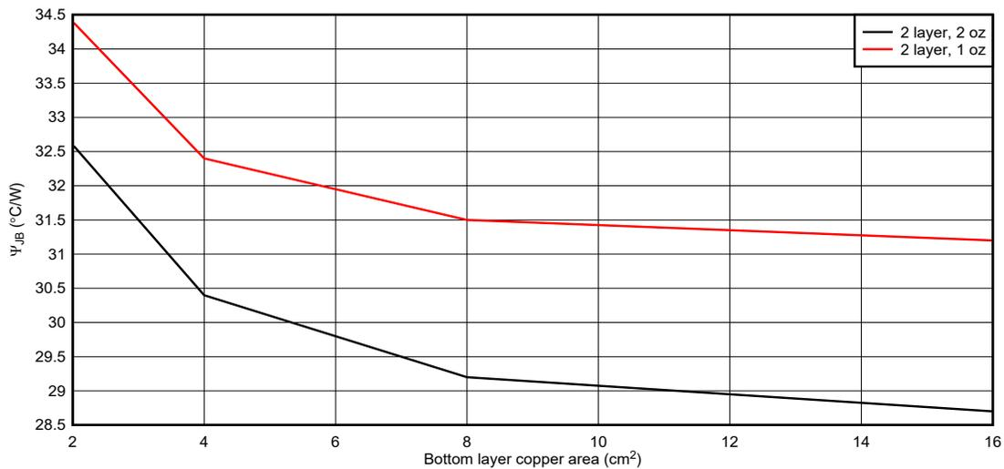
**Figure 9-16. WQFN, junction-to-board characterization parameter vs copper area**
