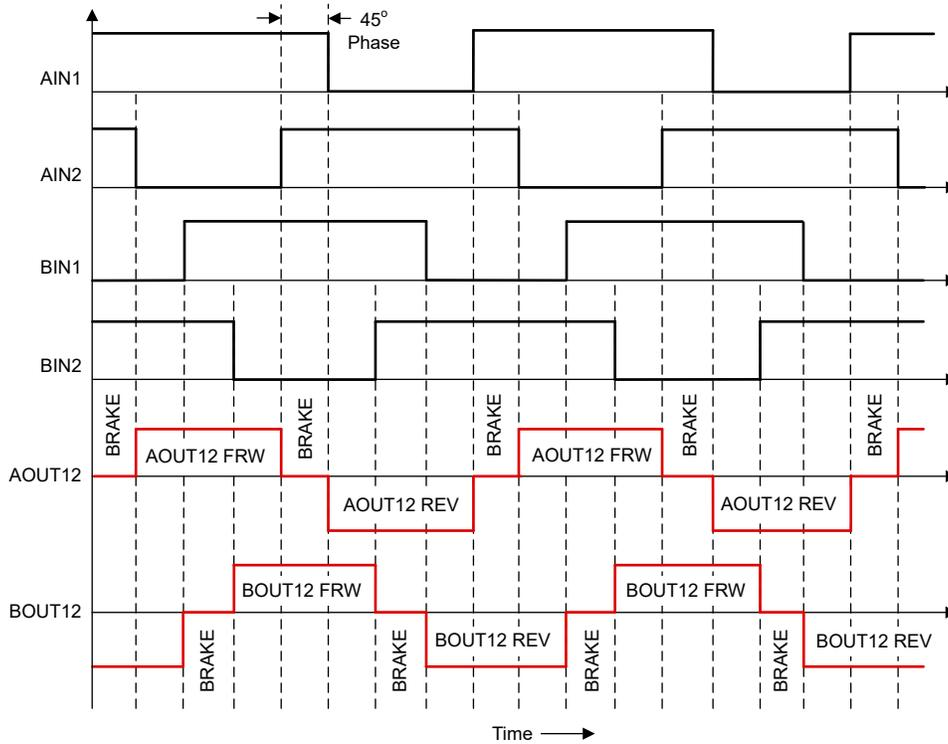
**Figure 9-4. Timing Diagram for Half-Stepping with Slow Decay**
