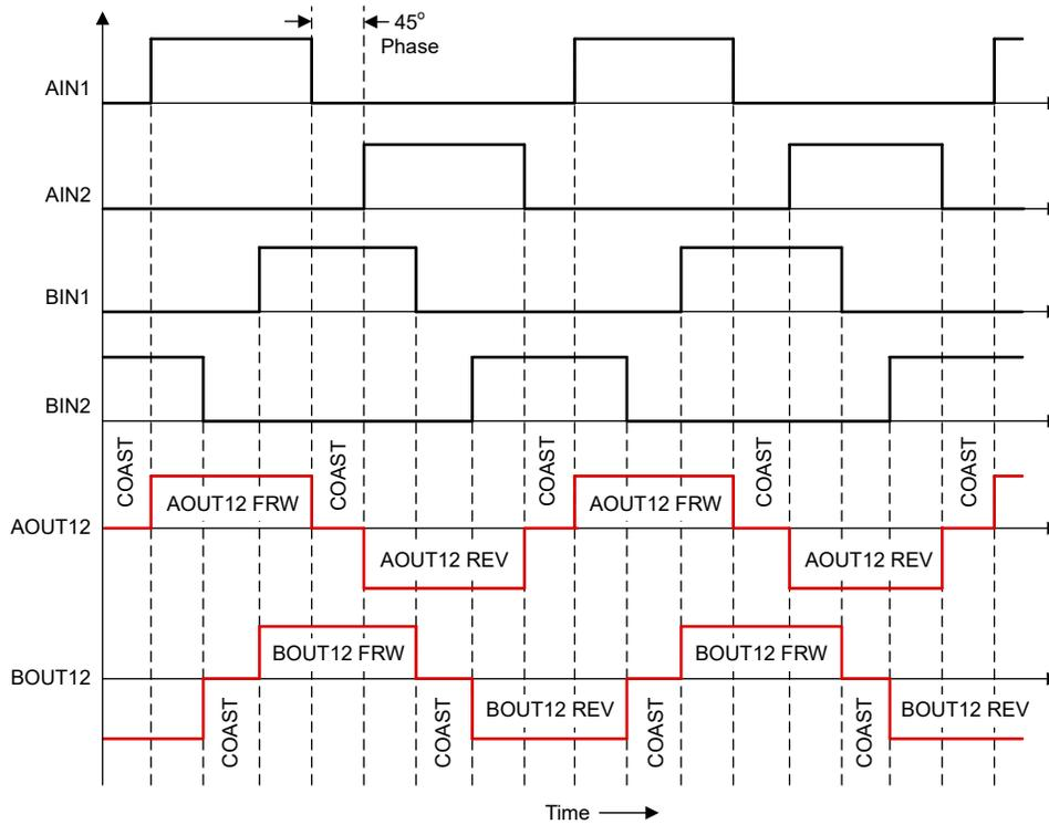
**Figure 9-3. Timing Diagram for Half-Stepping with Fast Decay**
