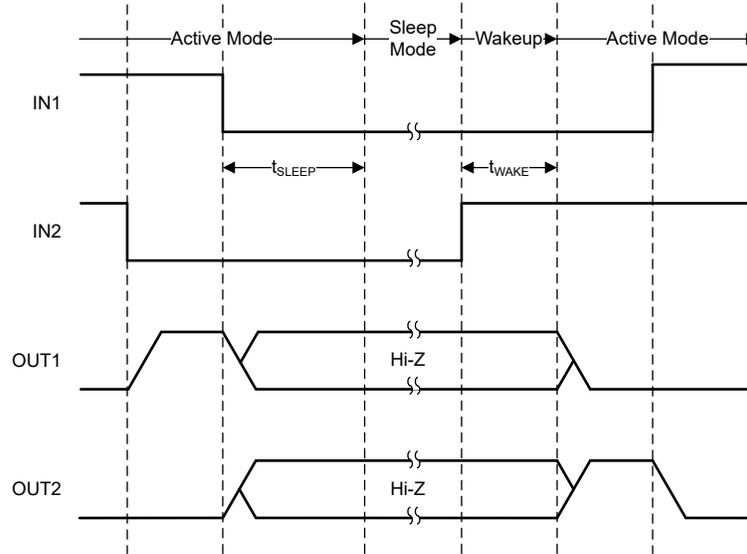
Figure 8-8. Sleep Mode Entry and Wakeup Timing Diagram
