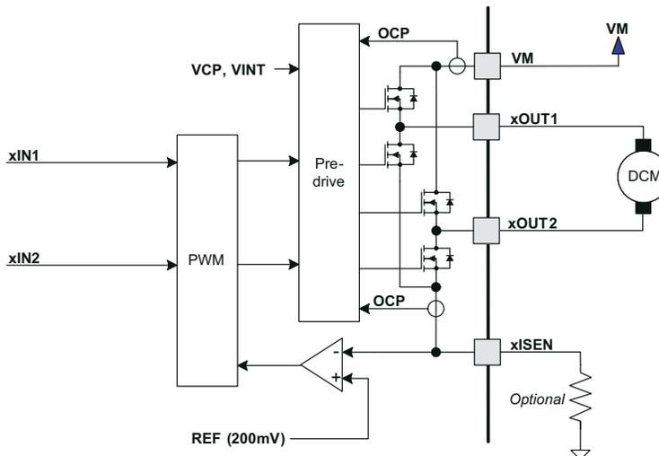
**Figure 8-4. Current Regulation Circuit**
