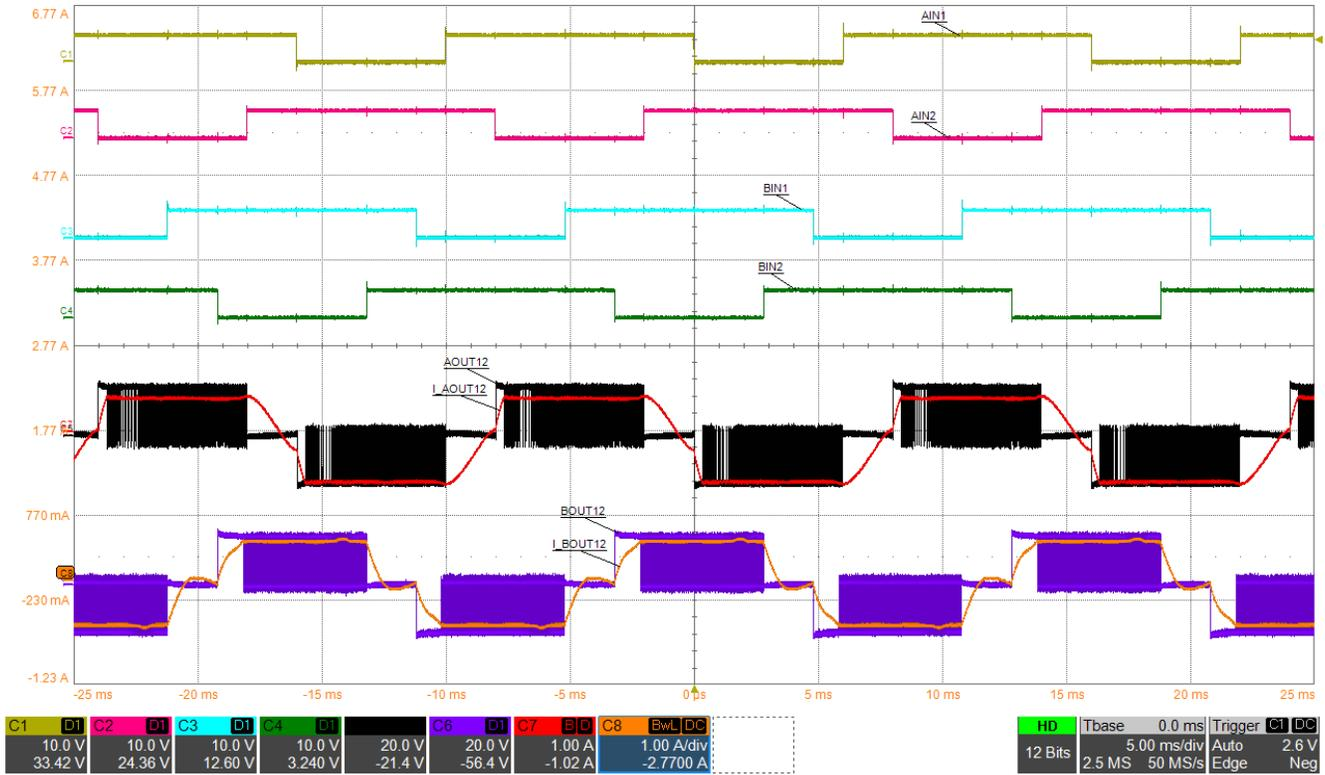
**Figure 9-7. Stepper Motor Half-Step Operation With Slow Decay**
