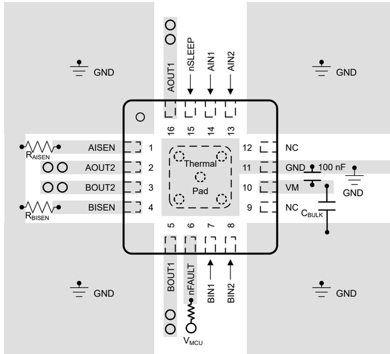
Figure 9-25. Recommended Layout Example for RTE (WQFN) Package
