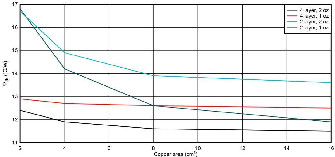
**Figure 9-14. HTSSOP, junction-to-board characterization parameter vs copper area**
