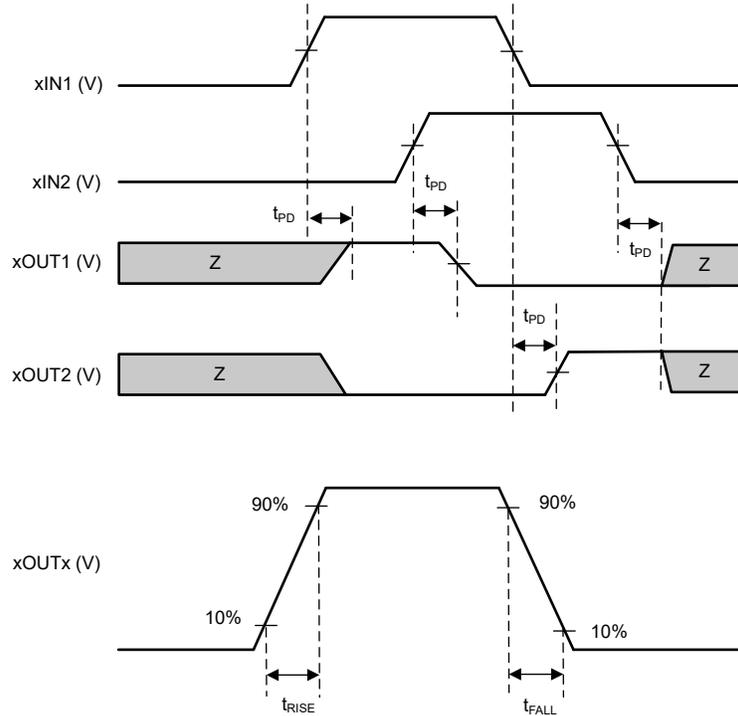
**Figure 6-1. Input-to-Output Timing**
