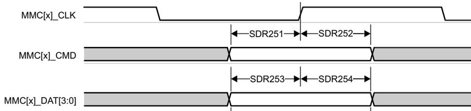
Figure 6-96. MMC1/MMC2 – UHS-I SDR25 – Receive Mode
