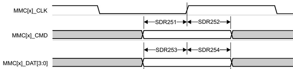
**Figure 6-85. MMC0 – UHS-I SDR25 – Receive Mode**
