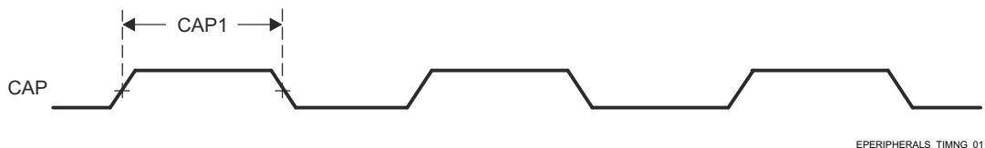
Figure 6-14. ECAP Timings Requirements
