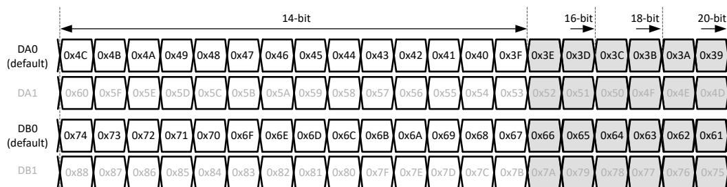
Figure 7-45. 1-wire output bit mapping
