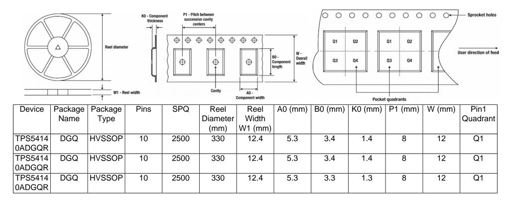
Images above are just a representation of the carrier. Actual carrier may vary. Please reference the dimensions provided in the table.
