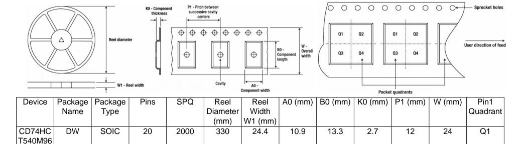
Images above are just a representation of the carrier. Actual carrier may vary. Please reference the dimensions provided in the table.
