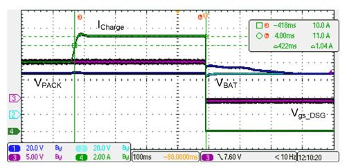
Figure 3-6. Overcurrent Charge
