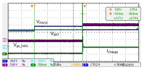
Figure 3-14. Standby Mode to Normal Mode (Charge)
