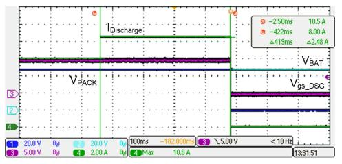
Figure 3-5. Level 1 Overcurrent Discharge
