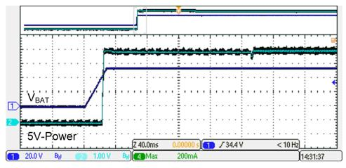
Figure 3-11. Shutdown Mode to Normal Mode
