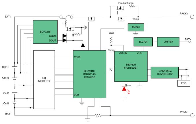
Figure 2-1. TIDA-010208 Block Diagram
