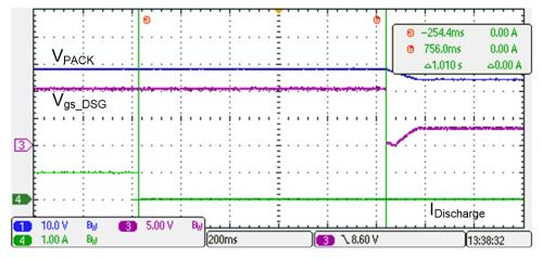
Figure 3-13. Normal Mode (Discharging) to Standby Mode
