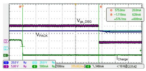
Figure 3-12. Normal Mode (Charging) to Standby Mode
