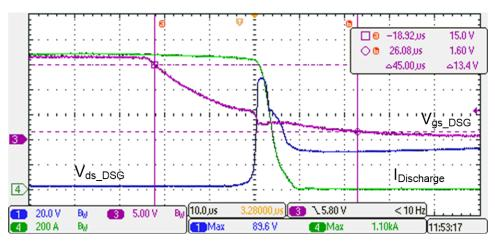
Figure 3-7. Discharge Short Circuit
