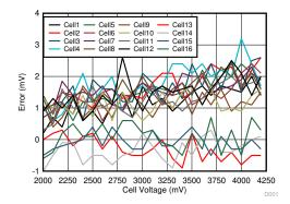
Figure 3-3. Cell Voltage Accuracy
