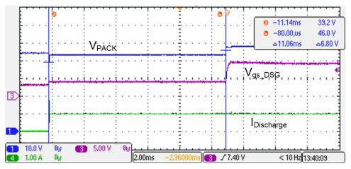
Figure 3-15. Standby Mode to Normal Mode (Discharging)
