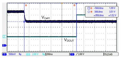
Figure 3-9. Secondary Undervoltage Protection
