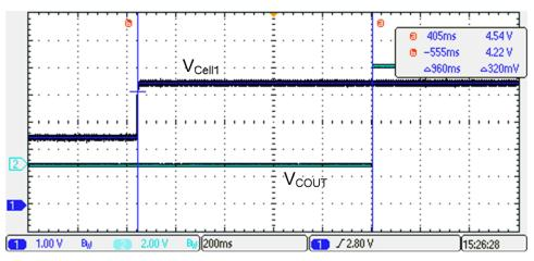
Figure 3-8. Secondary Overvoltage Protection
