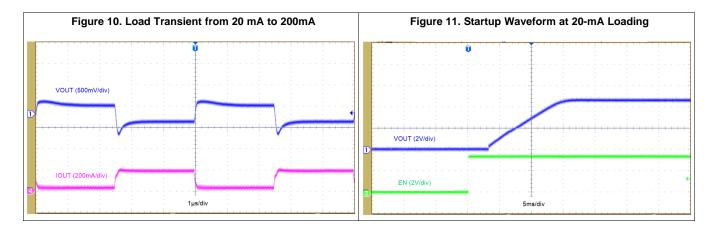
The startup waveform at 20mA loading condition is shown in Figure 11.
