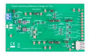
9 Multi-rail TV Power Supply Reference Design With Flexible Partitioning to Maximize Power Savings Copyright © 2019, Texas Instruments Incorporated
