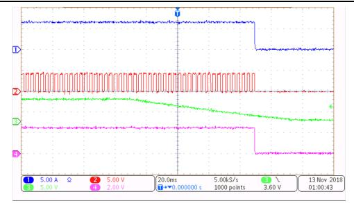
Figure 17. POL Enable Toggle Low With Phase Node
