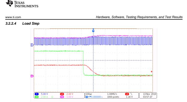
Figure 11. Negative Load Step With Phase Node
