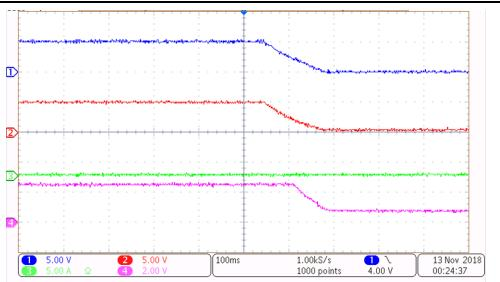
Figure 10. Shutdown Waveform No Load With Output Current
