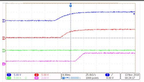
Figure 6. Start-up Waveform No Load With Output Current Node
