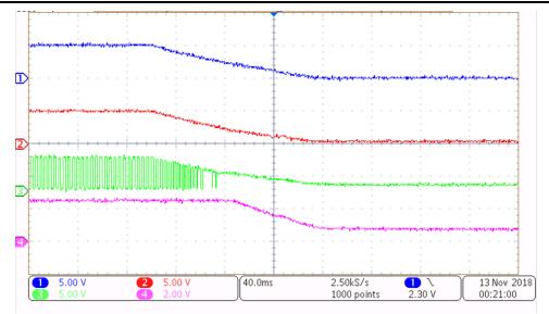
Figure 9. Shutdown Waveform No Load With Phase Node
