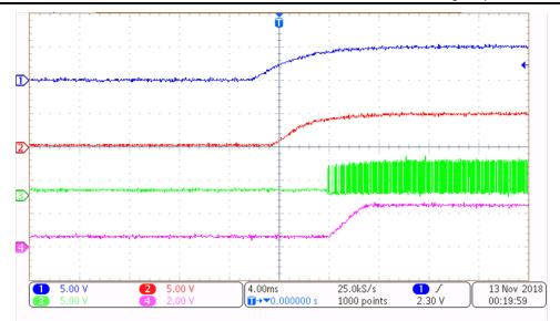
Figure 5. Start-up Waveform No Load With Phase Node
