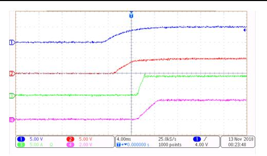
Figure 4. Start-up Waveform Full Load With Output Current
