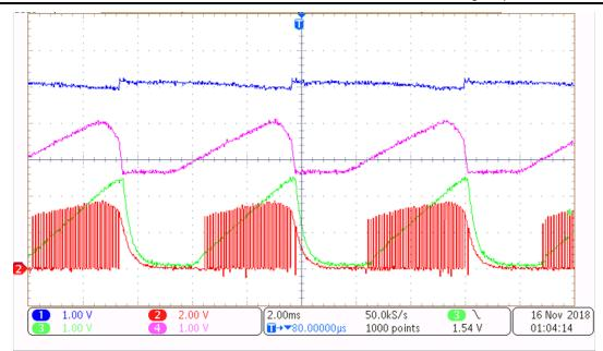
Figure 19. Load Switch Current Limit With Phase Node
