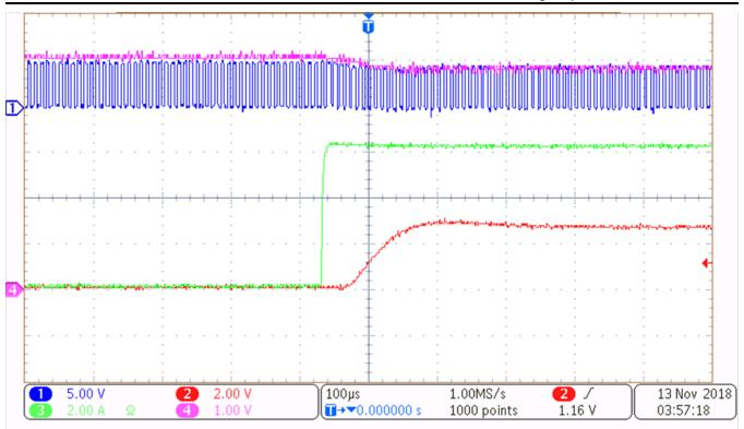
Figure 13. Positive Load Step With Phase Node
