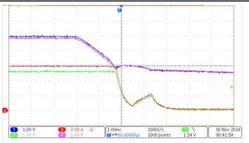
Figure 8. Shutdown Waveform Full Load With Output Current
