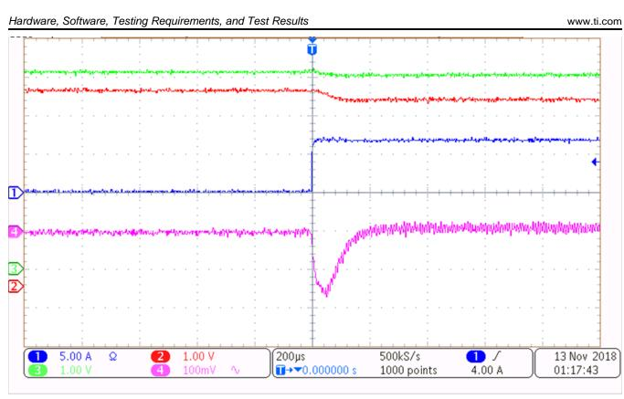
Figure 14. Positive Load Step With Input Voltage
