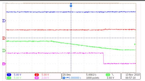
Figure 18. POL Enable Toggle Low With Input Voltage
