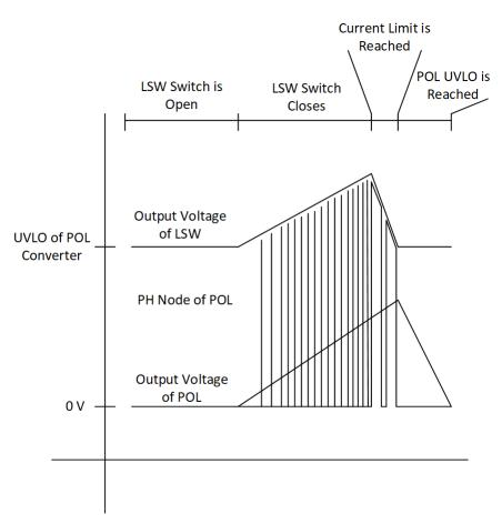
Figure 21. Breakdown of Load Switch Current Limit
