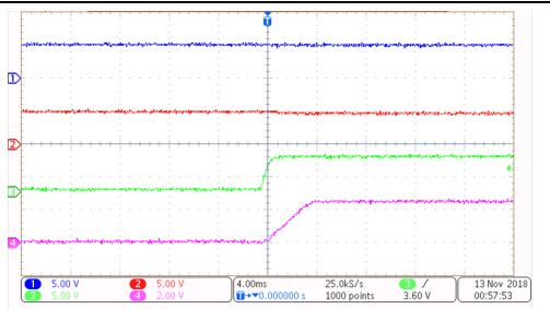
Figure 16. POL Enable Toggle High With Input Voltage
