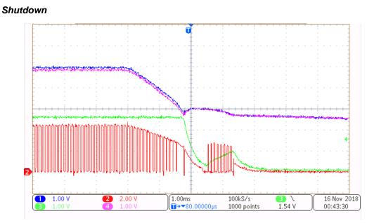
Figure 7. Shutdown Waveform Full Load With Phase Node
