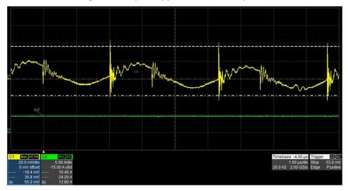
Figure 10. Input Ripple, 20 mV/div, 1 µs/div
