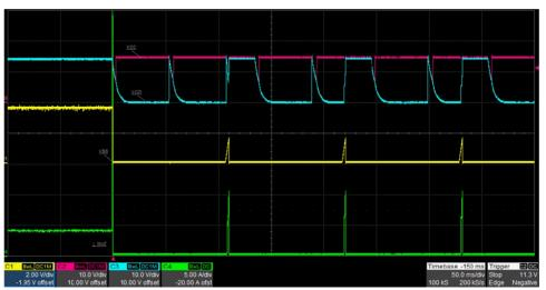
Figure 16. Short Circuit Hiccup Response, 50 ms/div
