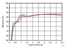
Figure 6. 48-V Efficiency for PoE, Adapter and DC/DC Converter
