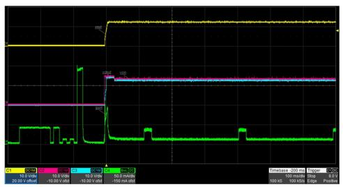
Figure 15. Startup Waveforms at 5-mA Load, 100 ms/div
