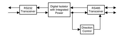
Figure 1. TIDA-060008 Block Diagram
