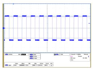
Figure 8. Input 1 kHz RS-232 clock data
