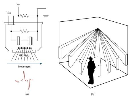
Figure 2. (a) Fresnel Lens, (b) Wedge-Shaped Sensory Patterns
