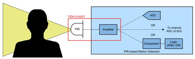
Figure 1. Typical Block Diagram of a PIR-Based Motion Detector Sub-System
