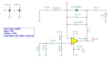
Figure 16. Test Circuit for Stage-1 Stability Analysis
