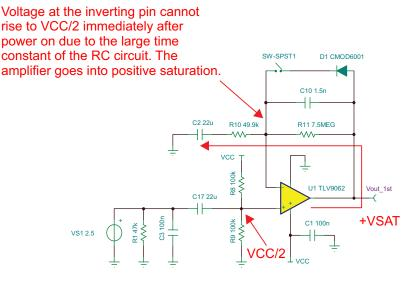
Figure 13. Power-on Settling Time Simulation Without Diode
