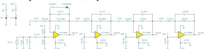
Figure 11. TINA Schematic for Settling Time Simulation With and Without Diode
