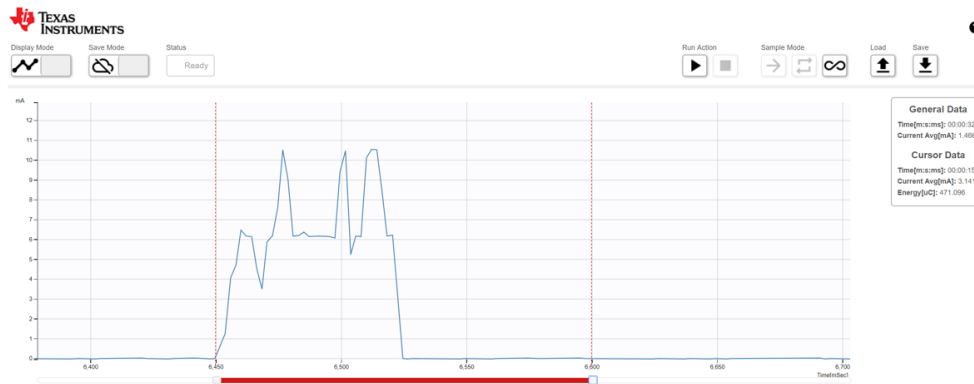
Figure 27. Sensor Current Consumption for Reception of 1-Byte Data
