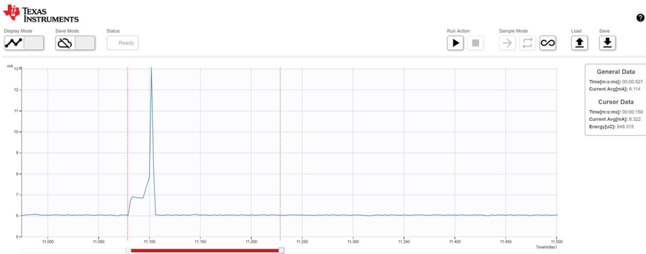
Figure 35. Collector Current Consumption for Receiving 70-Byte Data
