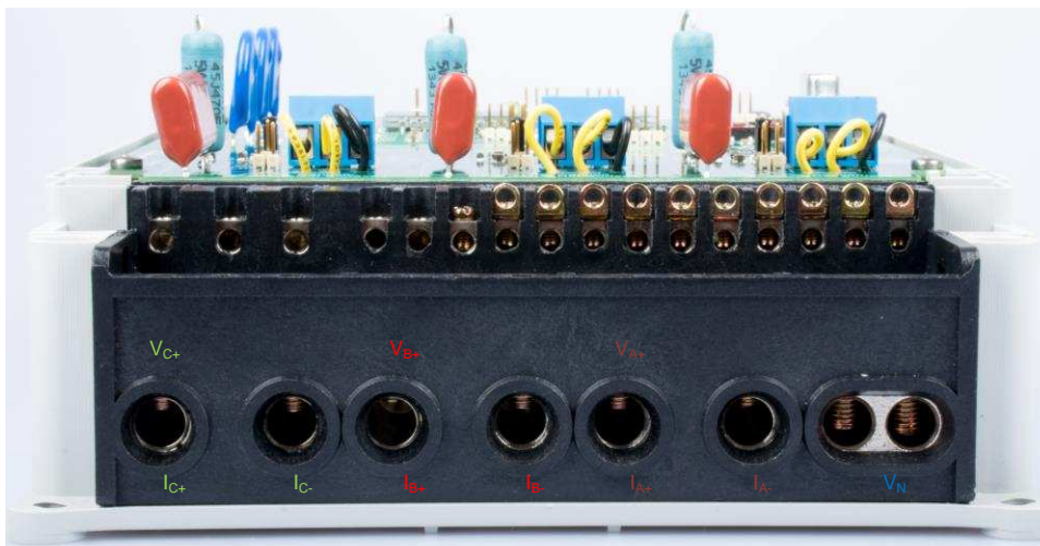
Figure 28. Front View of Reference Design with Test Setup Connections
