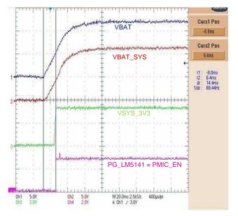
This appendix shows oscilloscope images of the initial power-up sequence of the TPS65916 PMIC.
