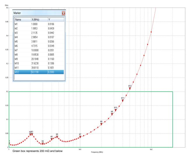
Figure 23. Target Impedance: VDD\_DDR\_1V35
