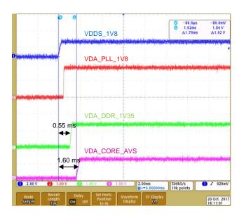
Figure 8. TPS65916 Stage 4 and 5 Power-up
