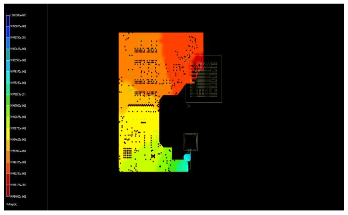
Figure 22. VDD\_DDR\_1V35 IR Drop Analysis
