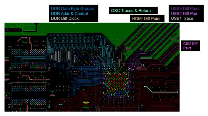
Figure 4. High-Speed Signaling Breakout Overview (Top Layer)
