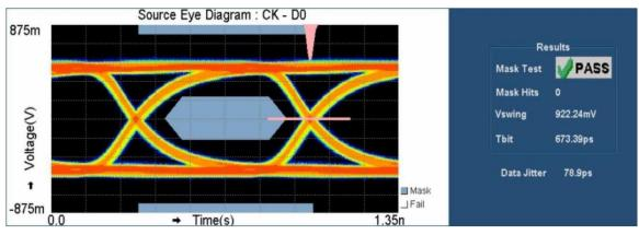
Figure 5. HDMI Eye Diagram Waveform
