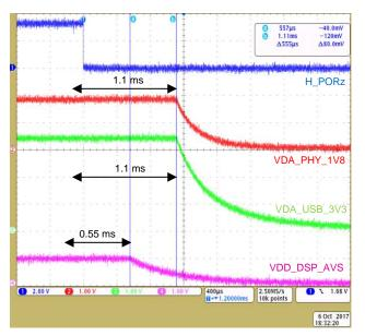
Figure 14. TPS65916 Stage 2 and 3 Power Down
