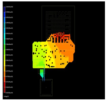
Figure 18. VDD\_DSP\_AVS IR Drop Analysis
