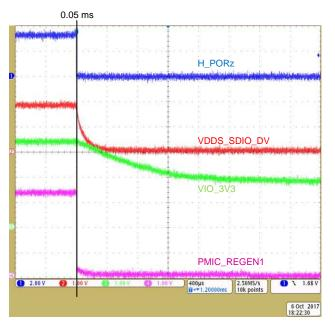
Figure 12. TPS65916 Stage 1 Power Down
