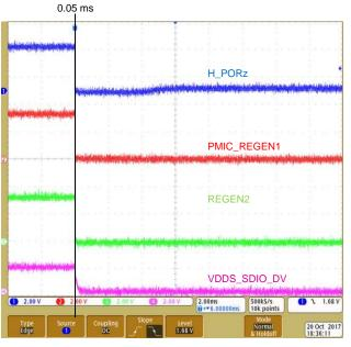
Figure 13. TPS65916 Stage 1 Power Down (Cont.)
