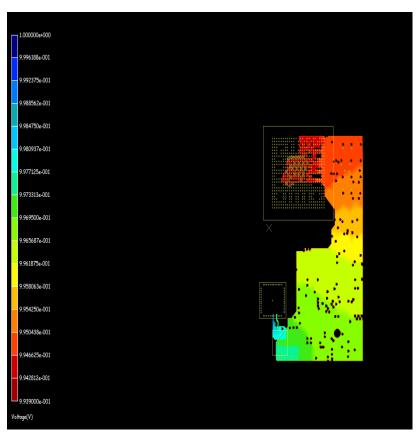
Figure 20. VDD\_CORE\_AVS IR Drop Analysis
