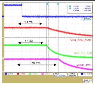
Figure 16. TPS65916 Stage 3 and 4 Power Down
