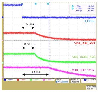
Figure 15. TPS65916 Stage 2 and 3 Power Down (Cont.)
