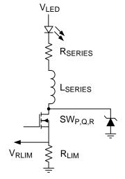
Figure 8. Parasitic Inductance (L<sub>series</sub>) and Resistance (R<sub>series</sub>) in Series With LED
