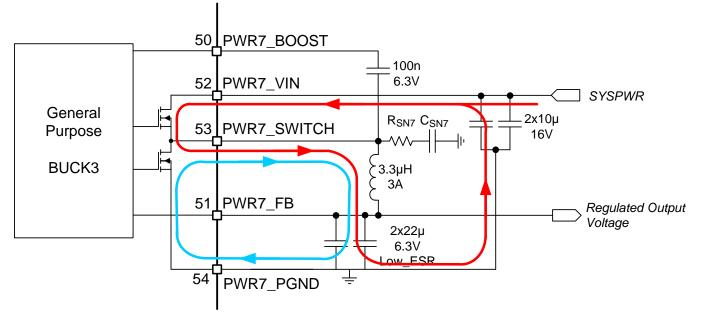
Figure 6. High AC Current Paths in a Buck Converter
