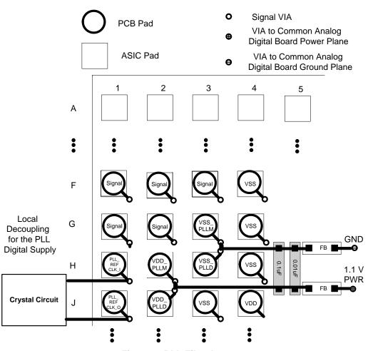
Figure 4. PLL Filter Layout
