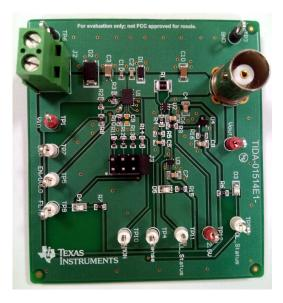
Protection and Light-Load Detection Reference Design for Antenna Module
