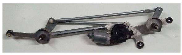
Figure 20. Front Wiper Hardware
