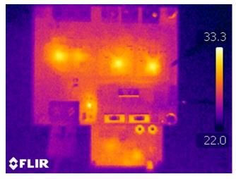
Figure 46. Infrared Image With Front Wiper Motor Active
