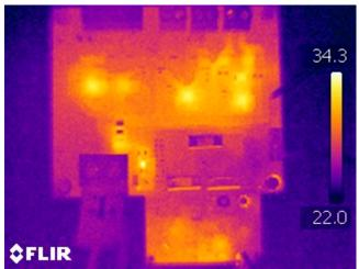
Figure 48. Infrared Image With Pump Motor Active
