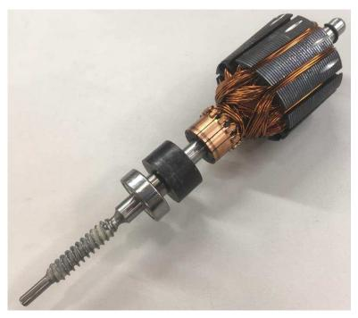
Figure 34. Detail of Typical Single-Speed Wiper Motor With Exposed Windings
