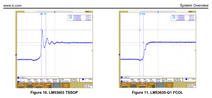
The difference between switch node ringing for a wire bond package and a HotRod package is illustrated in Figure 10 and Figure 11. The ringing overshoot is reduced from 9 V to 0 V, lowering the overall EMI and noise. Not only does the HotRod packaging help reduce EMI, but it also allows for a smaller size and reduced  $R_{DS ON}$ , improving efficiency.
