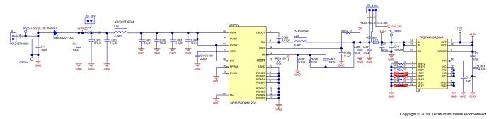
Figure 5. LM53635-Q1 Schematic
