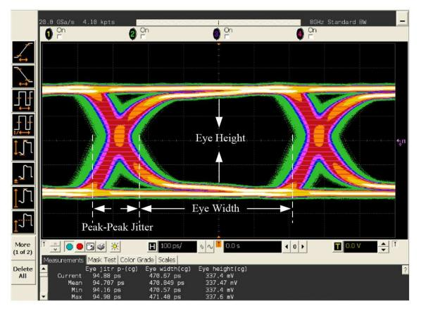
Figure 21. Setup Two Eye Diagram
