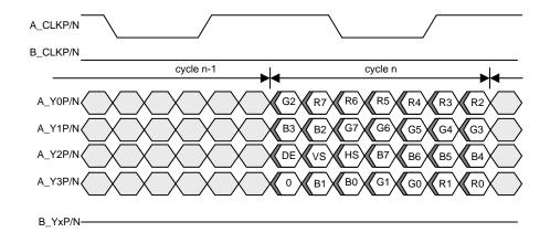
DE = Data Enable; Channel B Clock and Data are Output Low
