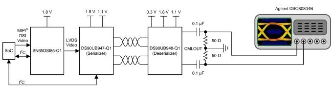
Figure 19. Eye Diagram Test Setup Two
