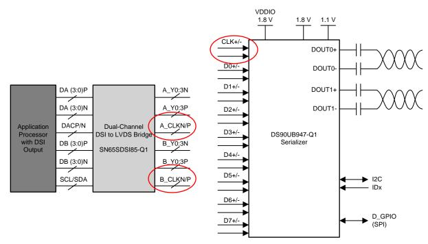
Figure 12. SN65DSI85-Q1 and DS90UB947-Q1 Connecting Considerations
