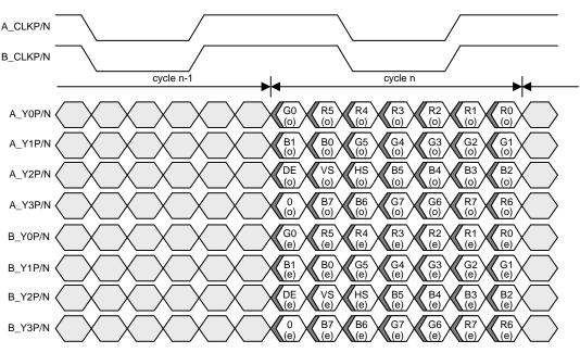
Figure 6. OLDI/LVDS Dual-Link 24-bpp Output Data (Format Two)
