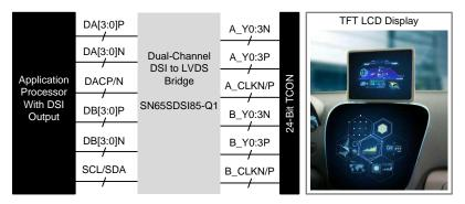
Figure 4. SN65DSI85-Q1 Typical Application
