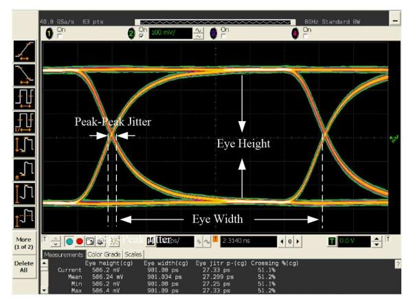
Figure 20. Setup One Eye Diagram
