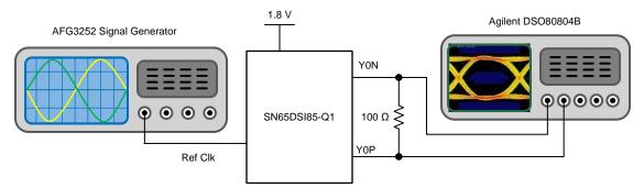
Figure 18. Eye Diagram Test Setup One
