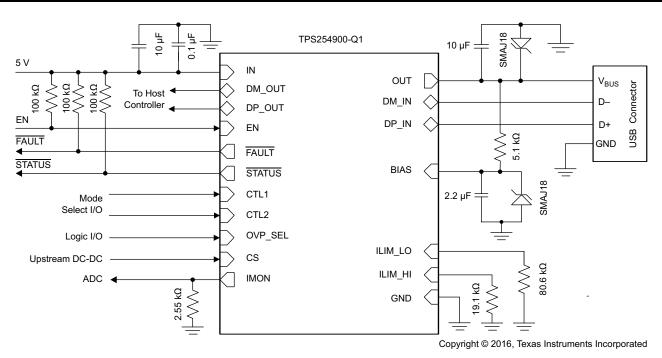
Figure 11. TPS254900-Q1 Simplified Circuit
