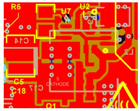
Figure 20. Reverse Battery Protection Layout
