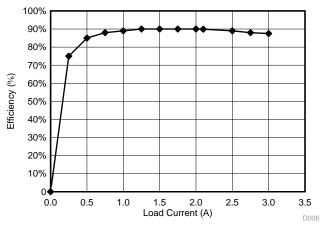
Figure 42.  $V_{IN}$  = 14.5 V Measured at C16 and LMS3635-Q1—Measured at COUT3
