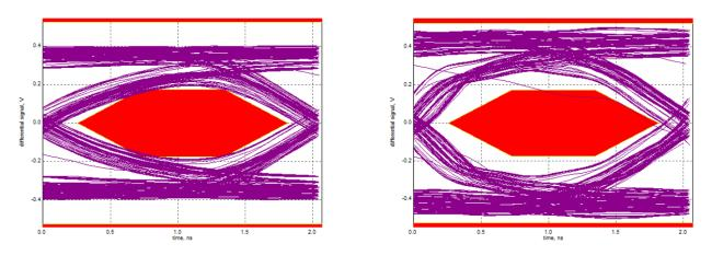
Figure 53. Far-End USB-IF Test With TUSB213-Q1 Disabled
