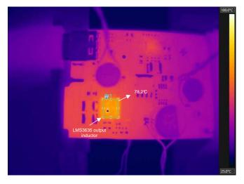
Figure 43. LMS3635-Q1 Output Inductor at 78.2°C:  $V_{IN}$  = 14.5 V,  $I_{LOAD}$  = 3 A, Soak Time = 20 min, Ambient Temperature 25°C
