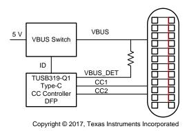
Figure 5. TUSB319-Q1 Simplified Circuit
