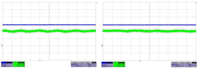
Figure 37.  $V_{IN}$  = 14.5 V Measured at C13 With No Load
