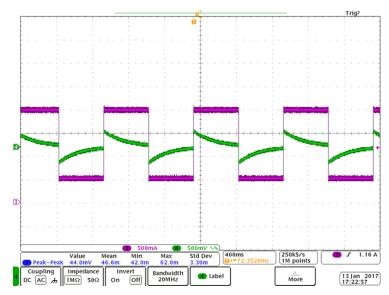
Figure 33. V<sub>IN</sub> = 13.5 V, Load Step = 0.5 A to 2 A (Switching), Load Transient = 250 mV at LMS3635 V<sub>OUT</sub> (COUT3)
