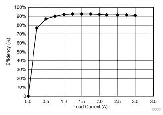
Figure 41.  $V_{IN}$  = 14.5 V Measured at C13 With TIDA-01432 Efficiency—Measured at COUT3
