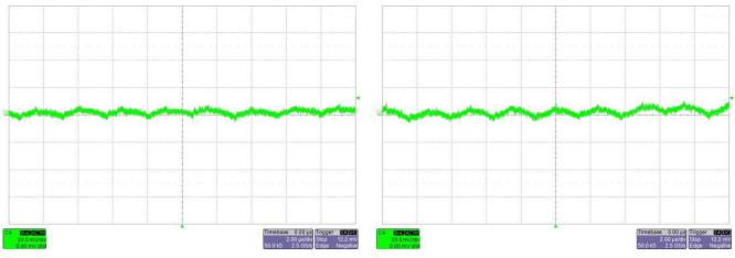
Figure 39.  $V_{IN}$  = 14.5-V Output Ripple Measured at COUT3 With No Load
