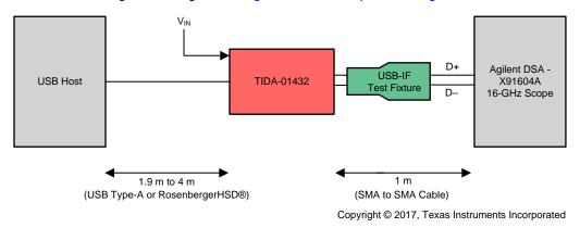
Figure 47. Block Diagram of Near-End Test Setup
