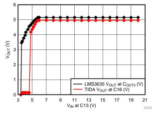
Figure 36.  $V_{IN}$  = 0 V to 20 V Measured at C13, 1.7- $\Omega$  Load
