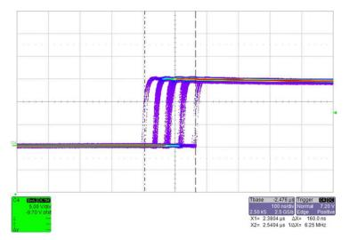
Figure 32. Spread Spectrum is ±3% of Switching Frequency
