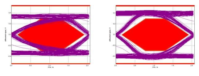
Figure 49. Near-End USB-IF Test With TUSB213-Q1 Disabled
