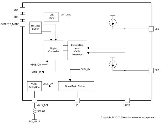
Figure 4. TUSB319-Q1 Functional Block Diagram
