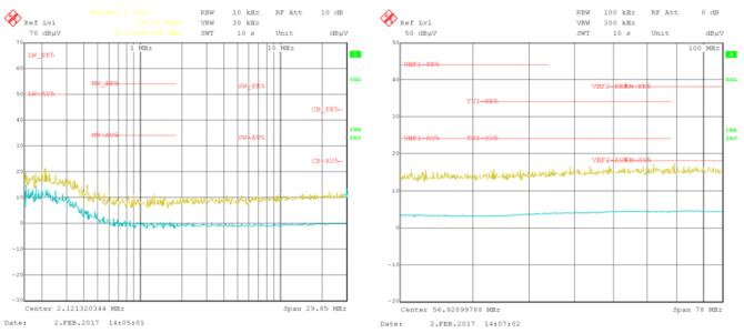
Figure 56. Low-Frequency Testing (100 kHz to 30 MHz) of Conducted EMI Performance
