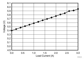
Figure 35.  $V_{IN}$  = 14.5 Measured at C13, USB  $V_{OUT}$ Measured at C16, Cable Compensation Enabled
