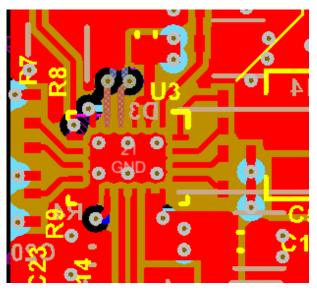
Figure 22. Legacy Charge Controller Layout
