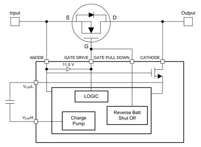
Figure 8. LM74610-Q1 Functional Block Diagram
