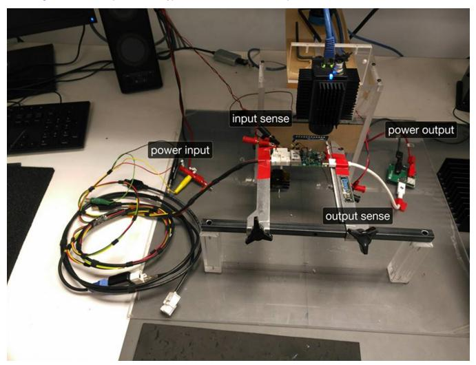
Figure 25. TIDA-01432—Typical Test Measurement Setup
