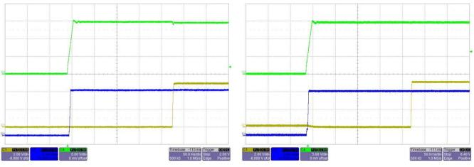
Figure 26. V<sub>IN</sub> = 14.5 V (Green), LMS3635 5 V<sub>OUT</sub> (Blue), USB 5 V (Yellow)—Start-Up = 15 ms at I<sub>OUT</sub> = 0 A
