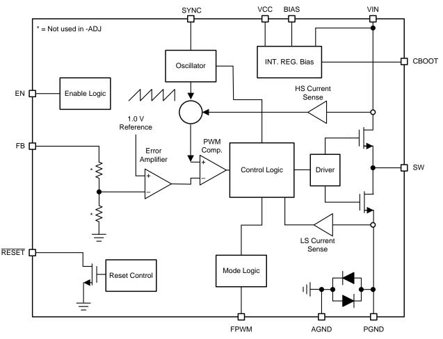
Figure 6. LMS3635-Q1 Functional Block Diagram
