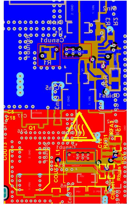
Note: The switch node is connected on the top and bottom of the board to minimize EMI and couple the thermals between the IC and inductor. A snubber and tuning resistor are also added.
