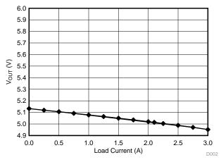
Figure 34.  $V_{IN}$  = 14.5 Measured at C13, USB  $V_{OUT}$  Measured at C16, Cable Compensation Disabled
