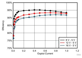
Figure 6. TIDA-01448 Efficiency
