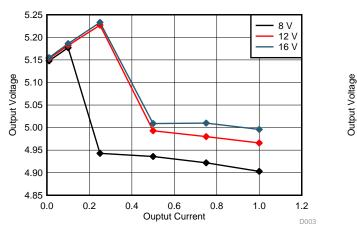
Figure 8. Line and Load Regulation at 85°C
