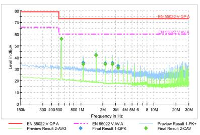
Figure 22. Conducted Emission Test Result
