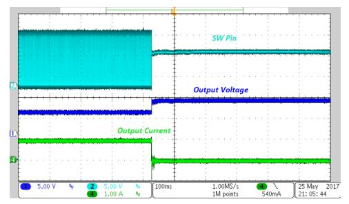
Figure 20. Overvoltage Protection From 5 to 6 V
