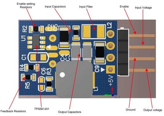
Figure 4. TIDA-01448 PCB With Functional Blocks
