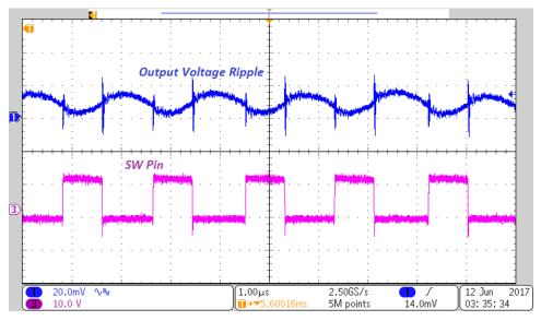
Figure 11. Output Voltage Ripple at 1-A Output Load
