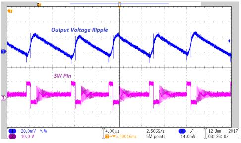
Figure 12. Output Voltage Ripple at 10-mA Output Load
