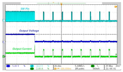
Figure 18. Overcurrent Protection
