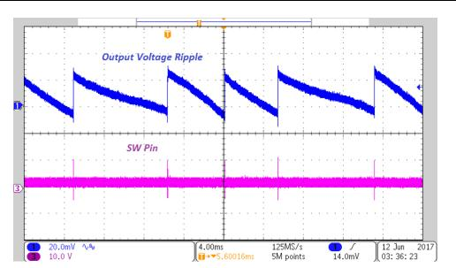
Figure 13. Output Voltage Ripple at No Load Output
