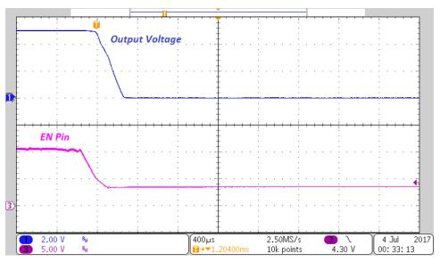
Figure 17. Shutdown at 12-V Input and 1-A Output Load
