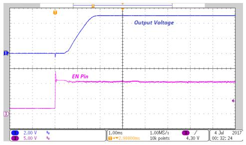
Figure 16. Start-up at 12-V Input and 1-A Output Load
