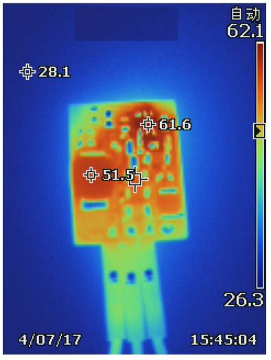
Figure 7. Top-Side Thermal Picture With 12-V<sub>IN</sub>, 5 V at 1-A Output
