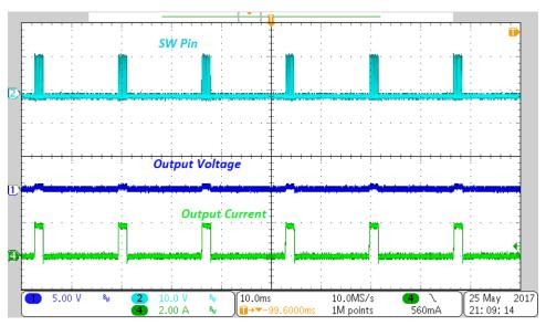
Figure 19. Short-Circuit Protection
