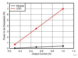
Figure 3. Comparison of Power Dissipated
