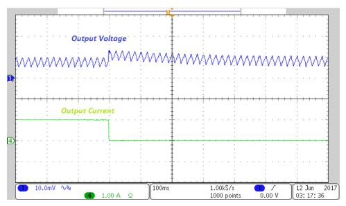
Figure 15. Transient Response From 1-A to 10-mA Output Load
