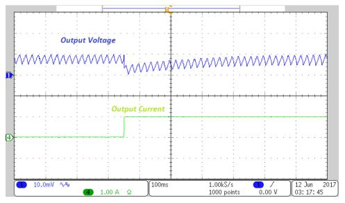
Figure 14. Transient Response From 10-mA to 1-A Output Load
