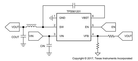
Figure 2. Block Diagram
