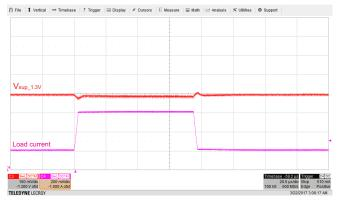
Figure 12.  $V_{sup_{-1.3V}}$  Transient Response (14 V<sub>IN</sub>, 400- to 800-mA Load Step, Measured at J6)
