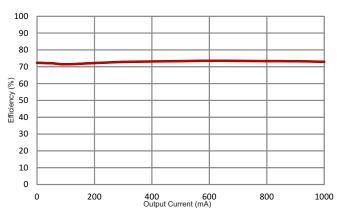
Figure 10.  $V_{sup_{-1.3V}}$  Efficiency (14  $V_{IN}$ , Measured at J6)
