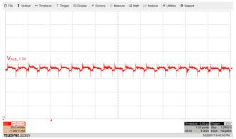
Figure 13.  $V_{sup\_1.3V}$  Ripple (14  $V_{\text{IN}}$  500-mA load on  $V_{sup\_1.3V}$  , 500-mA load on  $V_{sup\_5V}$  , Measured at J6)
