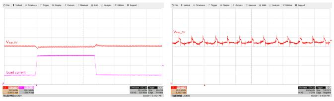
Figure 4.  $V_{sup_{.5V}}$ Transient Response (14 V<sub>IN</sub>, 400-mA to 800-mA Load Step, Measured at J4)
