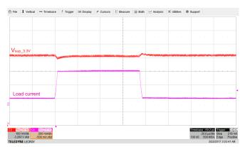
Figure 8.  $V_{sup_{.33V}}$  Transient Response (14  $V_{IN}$ , 100-mA to 500-mA Load Step, Measured at J5)
