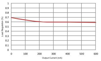
Figure 7.  $V_{sup_{-3.3V}}$  Load Regulation (14  $V_{IN}$  , Measured at J5)
