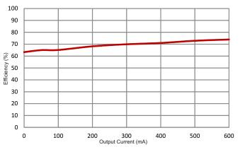
Figure 6.  $V_{sup_{3.3V}}$  Efficiency (14  $V_{IN}$ , Measured at J5)
