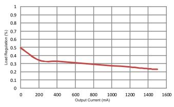
Figure 3.  $V_{sup_{5V}}$  Load Regulation (14  $V_{IN}$ , Measured at J4)
