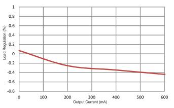
Figure 11.  $V_{\text{sup}\_1.3V}$  Load Regulation (14  $V_{\text{IN}}$ , Measured at J6)
