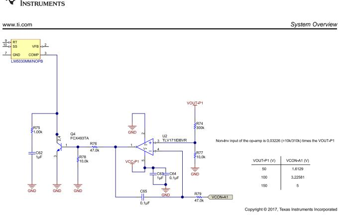
Figure 14. Feedback Circuit for Positive Rail for HV Section
