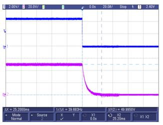
Figure 77. +LV/Mid-Out (Turnoff) From 50 to 0 V at Full Load
