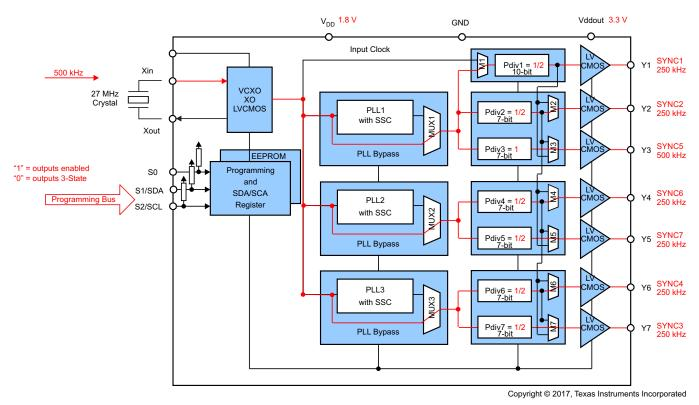
Figure 42. Clock Programming for Synchronization of All Devices to  $f_{IN}$  = 500 kHz
