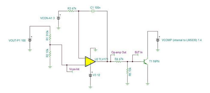
Figure 15. TINA Simulation for Feedback Circuit for Positive Rail for HV Section
