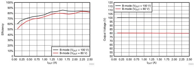
Figure 44. B-Mode Efficiency (+HV Output)
