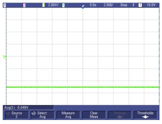
Figure 92.  $V_{out} = -5 V$  at  $V_{IN} = 24 V$
