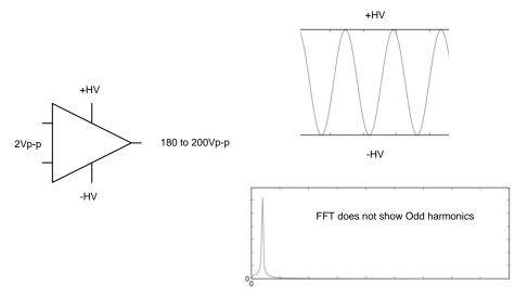
Figure 5. Linear Amplifier—Output Waveform and FFT of Output
