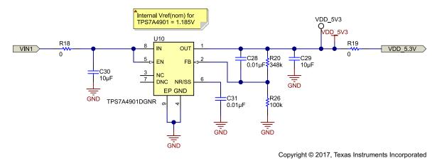
Figure 27. Power Supply for DAC60004
