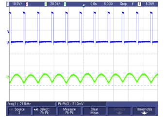
Figure 89. SW Node Waveform and Output Ripple for  $V_{out} = 3.3 \text{ V}$ ,  $I_{out} = 1 \text{ A}$
