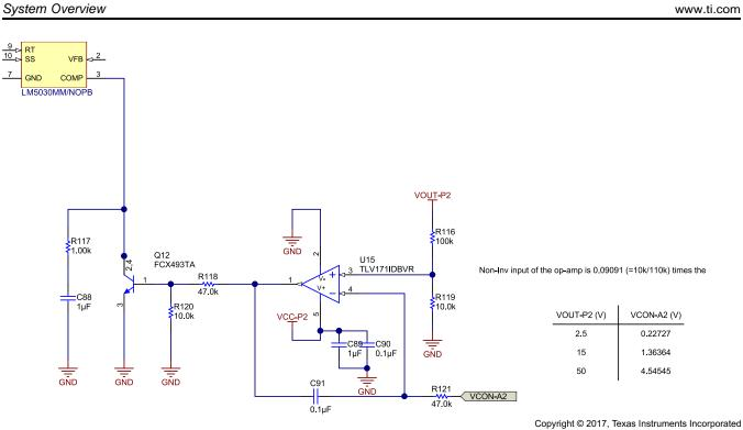
Figure 20. Feedback Circuit for Positive Rail for LV or MID Section
