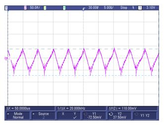
Figure 52. Output Voltage Ripple for +HV Output
