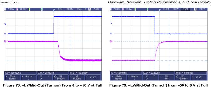
Figure 78. –LV/Mid-Out (Turnon) From 0 to –50 V at Full Load
