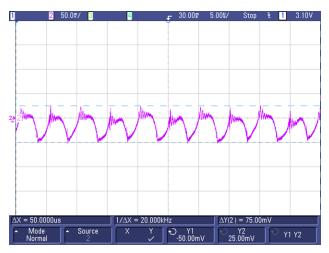
Figure 61. Output Voltage Ripple for -HV Output
