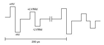
Figure 7. Five-Level Pulser Output Waveform
