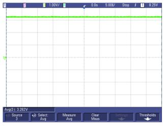
Figure 87.  $V_{out}$  = 3.3 V at  $V_{IN}$  = 24 V
