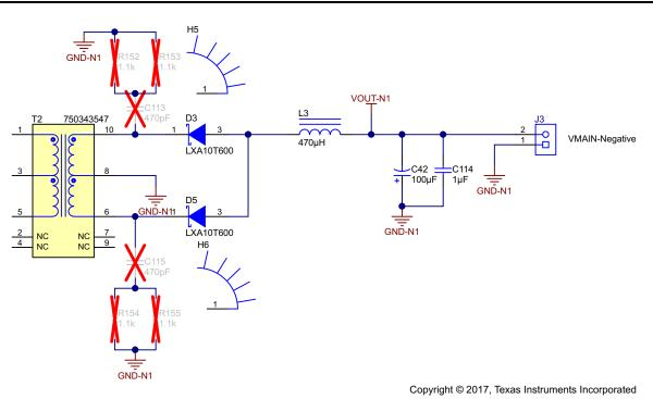
Figure 13. Output Rectifier and Filtering for Negative Output
