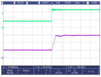
Figure 72. +HV-Out (Turnon) From 50 to 150 V at Full Load
