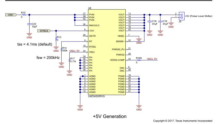
Figure 29. 5-V Generation Using LMZ34202
