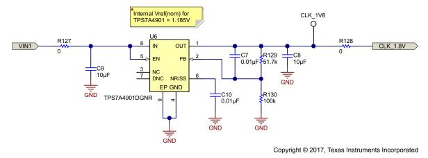
Figure 35. 1.8-V VDD Generation for CDCE937
