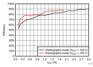
Figure 55. Elastography Mode Efficiency (-HV Output)
