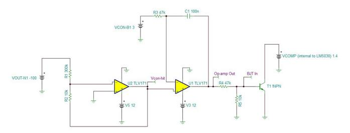
Figure 18. TINA Simulation for Feedback Circuit for Negative Rail for HV Section
