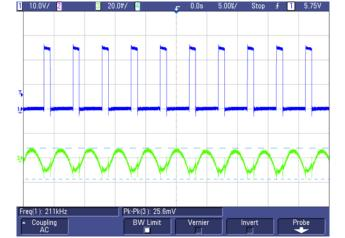
Figure 84. SW Node Waveform and Output Ripple for  $V_{out} = 5 V$ ,  $I_{out} = 1 A$
