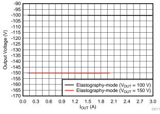
Figure 56. Elastography Mode Load Regulation (-HV Output)
