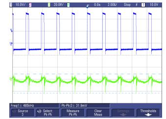
Figure 94. SW Node Waveform and Output Ripple for  $V_{out} = -5 V$ ,  $I_{out} = -1 A$
