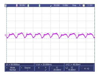
Figure 67. Output Voltage Ripple for -LV or MID Output at Full load
