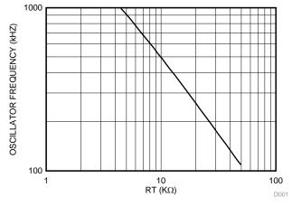
Figure 9. LM5030 Oscillator Frequency versus RT
