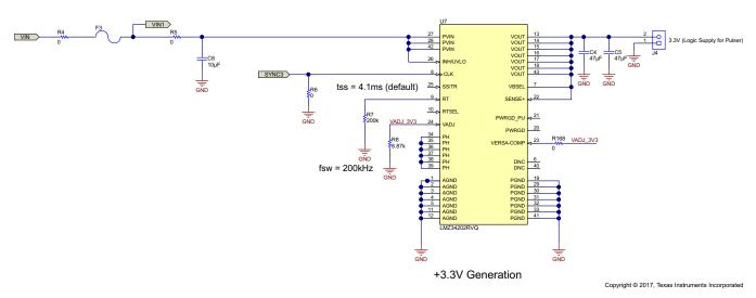
Figure 30. 3.3-V Generation Using LMZ34202
