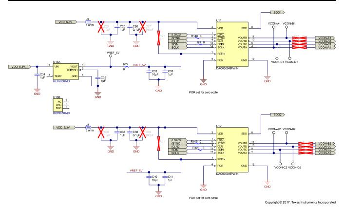
Figure 26. DAC60004 to set up Outputs for Power Supplies
