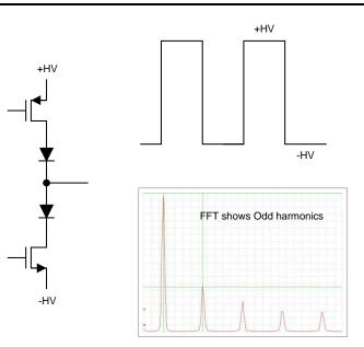
Figure 4. Pulser—Output Waveform and FFT of Output
