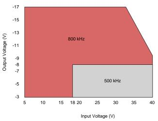
Figure 32. Recommended Switching Frequency for LMZ34002
