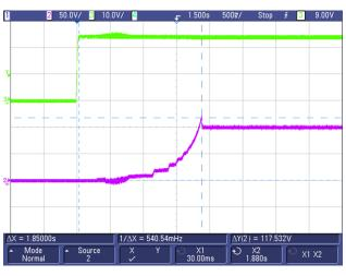
Figure 50. Start-up Waveform for +HV Output
