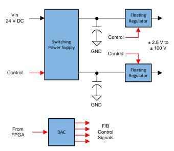
Figure 3. Typical Power Supply Scheme in Medical Ultrasound Application
