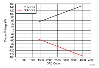
Figure 68. Output Voltage Linearity for U11 With Respect to Digital Input Code
