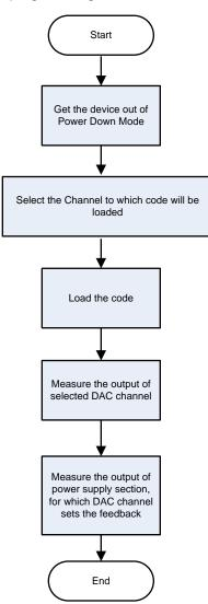
Figure 40. Flow Chart for Programming CDCE937
