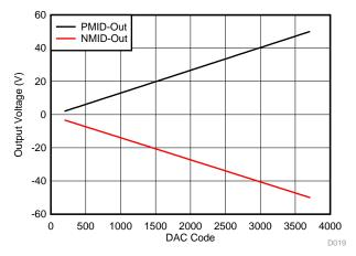
Figure 69. Output Voltage Linearity for U12 With Respect to Digital Input Code
