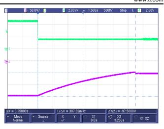
Figure 75. –HV-Out (Turnoff) From –150 to –50 V) at Full Load
