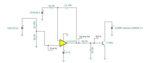
Figure 21. TINA Simulation for Feedback Circuit for Positive Rail for LV or MID Section
