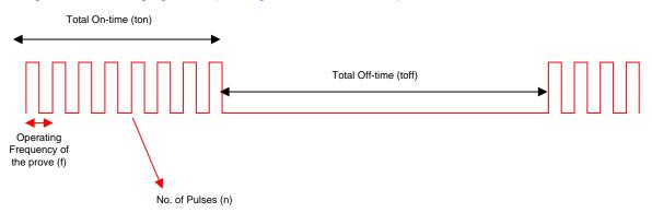
Figure 43. Load Profile for Testing TIDA-01352 in Different Imaging Modes
