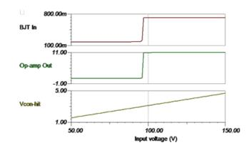
Figure 16. Simulation Waveform Showing Linearity (+HV Output)
