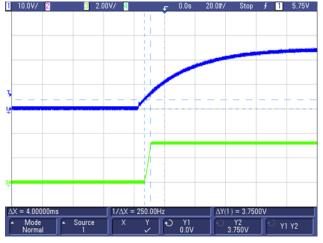
Figure 88. Start-up Waveform (for  $V_{out} = 3.3$  V) Showing Soft-Start Time = 4 ms
