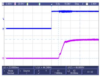
Figure 76. +LV/Mid-Out (Turnon) From 0 to 50 V at Full Load
