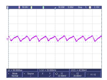
Figure 64. Output Voltage Ripple for +LV or MID Output at Full load
