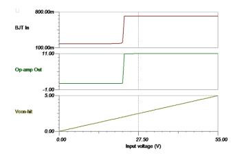
Figure 22. Simulation Waveform Showing Linearity (+LV or MID Output)
