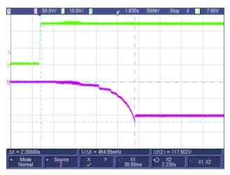
Figure 59. Start-up Waveform for -HV Output
