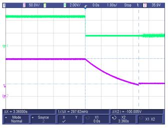
Figure 73. +HV-Out (Turnoff) From 150 to 50 V at Full Load
