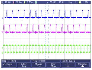
Figure 97. External SYNC Clock = 300 kHz (Channel 3 in Green)
