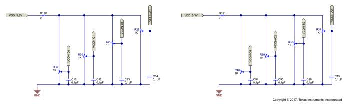
Figure 28. Potentiometers for Setting Feedback Outputs
