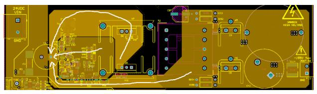
Figure 101. Star Ground Topology for Power Supply
