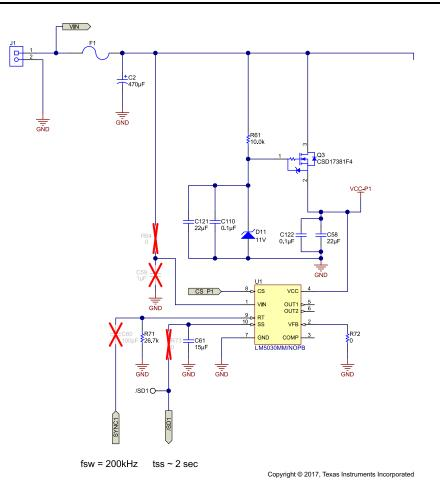
Figure 8. Input Section and Turnon Mechanism for LM5030
