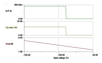
Figure 19. Simulation Waveform Showing Linearity (-HV Output)
