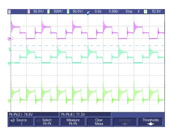
Figure 51. MOSFET Stress VDS for +HV Output
