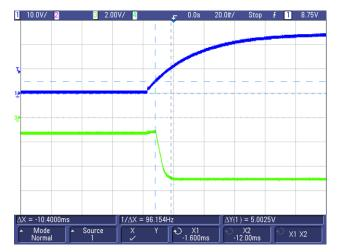
Figure 93. Start-up Waveform (for  $V_{out} = -5$  V) Showing Soft-Start Time = 10.4 ms
