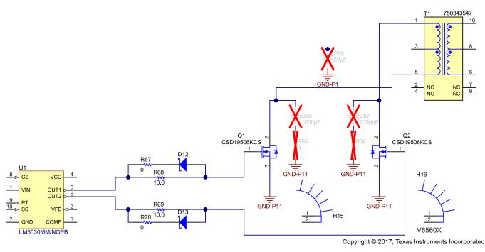
Figure 10. LM5030 Driving MOSFETs
