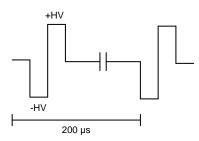
Figure 6. Three-Level Pulser Output Waveform
