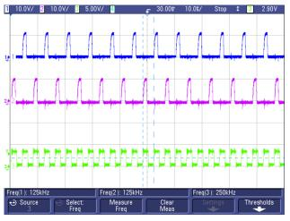
Figure 96. External SYNC Clock = 250 kHz (Channel 3 in Green)
