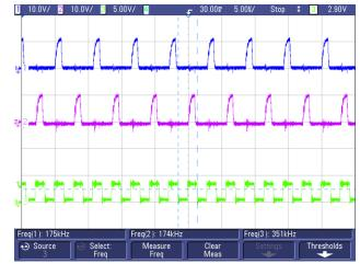
Figure 98. External SYNC Clock = 350 kHz (Channel 3 in Green)
