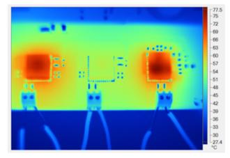
Figure 95. Thermal Image for LMZ Modules at Full Load
