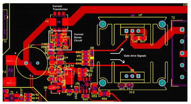
Figure 102. Routing for CS Pin for LM5030
