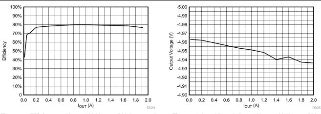
Figure 90. Efficiency at V<sub>IN</sub> = 24 V, V<sub>OUT</sub> = -5 V, I<sub>OUT</sub> = -2 A
