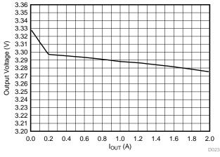
Figure 86. Load Regulation at  $V_{IN} = 24 V$ ,  $V_{OUT} = 3.3 V$
