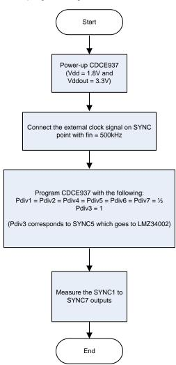
Figure 41. Flow Chart for Programming CDCE937
