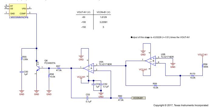
Figure 17. Feedback Circuit for Negative Rail for HV Section
