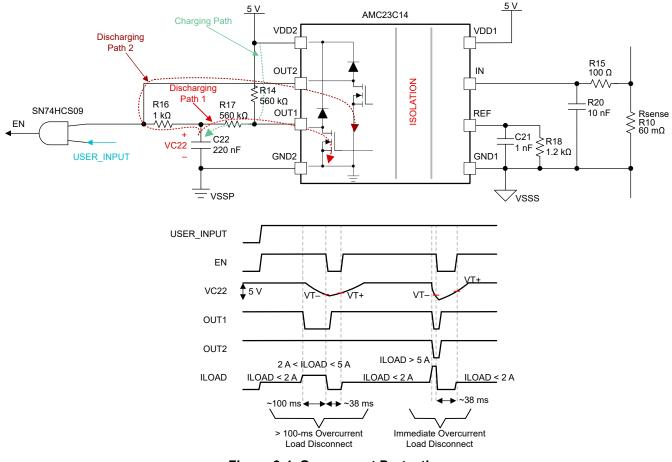
Figure 2-4. Overcurrent Protection
