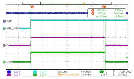
Figure 3-2. Scope Capture for 100-ms Delay Load Disconnect
