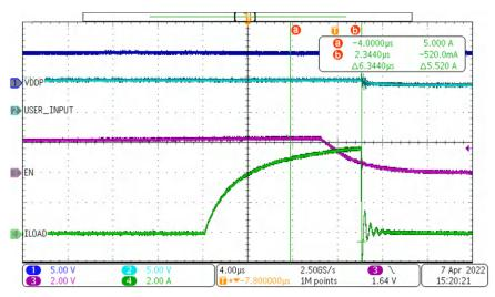
Figure 3-3. Scope Capture for Immediate Load Disconnect
