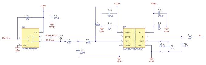
Figure 2-3. Overcurrent Detection Circuit
