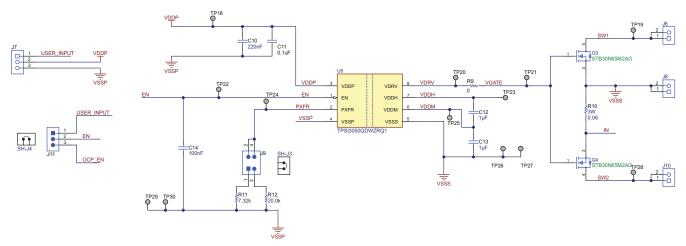
Figure 2-2. Solid-State Relay Circuit
