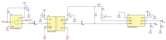
Figure 2-5. Overtemperature Detection Circuit
