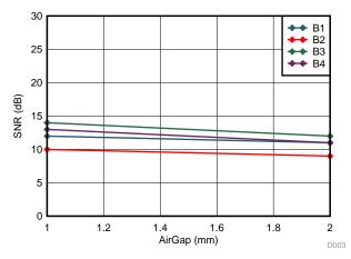
Figure 22. Finger Touch With Gloves—SNR
