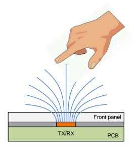
Figure 7. Self Capacitive Button Designs Example
