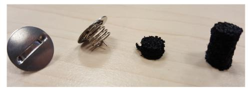
Figure 25. Springs and Filler Material
