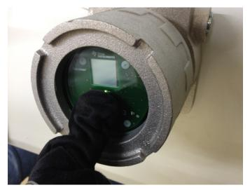
Figure 21. Touch With Gloves Test
