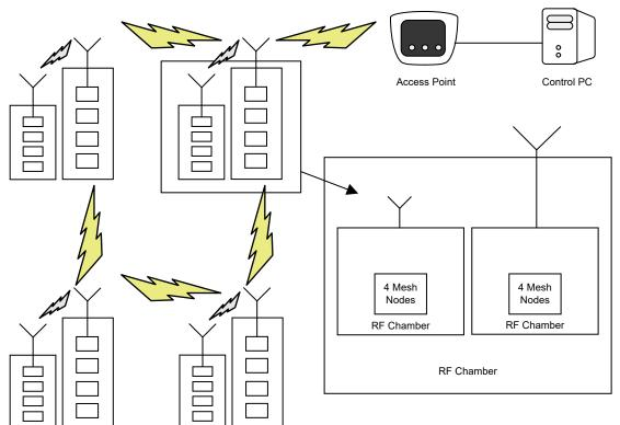
Figure 11-2. WiLink™ 8 32 Mesh Nodes Test Setup Illustration
