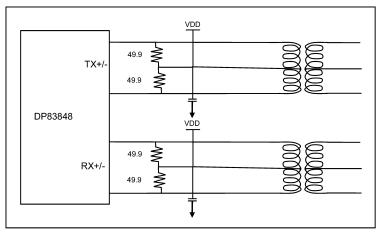
Figure 2. DP83848C/I/YB PMD Connections (Termination)
