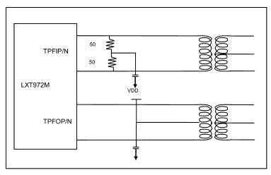
Figure 3. LXT972M PMD Connections (Termination)
