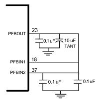
Figure 1. Special Connection in DP83848C/I/YB
