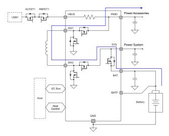
*Figure 3.* USB Type-C<sup>™</sup> FRS realized by single buck-boost charger.
