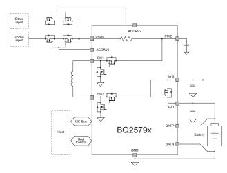
Figure 2. Example of a fully integrated buck-boost charger.
