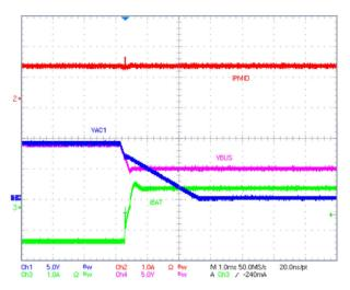
*Figure 4.* Buck-boost charger FRS from VBUS sink to VBUS source.
