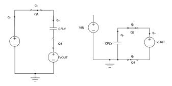
*Figure 2.* Capacitor and switches charge flow: charging, phase 1 (a); discharging, phase 2 (b).
