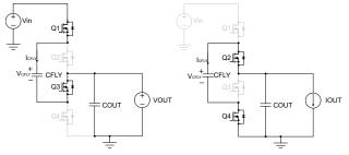
It is possible to use an ideal transformer in series with the output impedance (ROUT) to model the switchedcapacitor converter efficiency [3], including the chargesharing loss of the flying capacitor and the conduction loss in the resistive components. Switching loss is not included in the model, however, and requires separate analysis.
