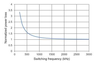
*Figure 3. Output impedance power loss of the 2-to-1 switchedcapacitor converter.*
