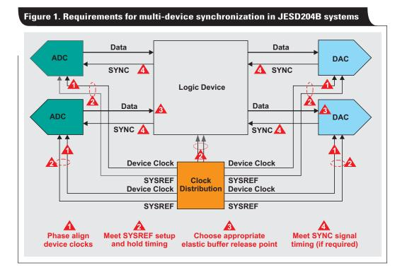
converter. The alignment of the device clocks is dependent on how well the propagation delays on the clock distribution paths are controlled, including how well the alignment is maintained over temperature changes.
