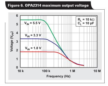
the mismatches between the amplifier rise and fall times and the responsivity of the amplifier at the peaks and valleys of the sinusoidal input voltage swing.
