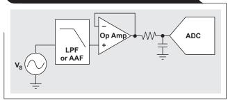
The DAQ system starts with a signal, such as a waveform from a sensor, V<sub>S</sub>. Next is the low-pass filter (LPF) or anti-aliasing filter (AAF) and the operational amplifier (op amp) configured as a buffer. At the output of the buffer amplifier is a resistor/capacitor pair that drives the ADC's input. The ADC is a successive-approximationconverter ADC (SAR ADC).
