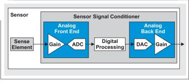
After the data from the front end is conditioned by the digital circuitry, it is sent to the back end for transmission to a control or monitoring system. The transmission of the conditioned signal can occur in either analog or digital form. In order to transmit the conditioned digital signal in analog form, a digital-to-analog converter (DAC) with a buffer or gain stage converts the digital value into analog form. Again, the PGA400-Q1 is an example of this type of signal conditioner.
