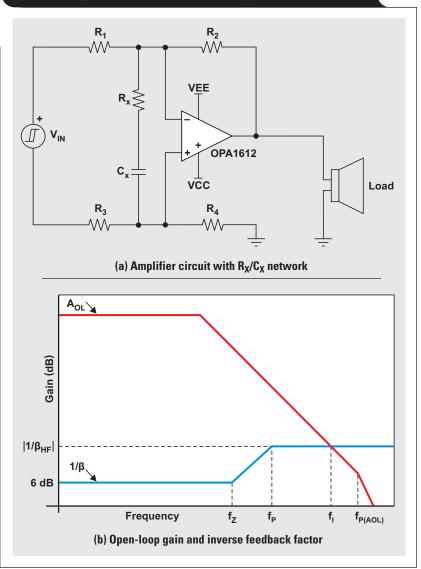
pair in the  $1/\beta$  curve. By increasing the magnitude of  $1/\beta$  at the frequency where it intersects the open-loop gain curve ( $f_I$ ), the system can achieve reasonable phase margin without increasing the output impedance at audio frequencies or degrading the CMRR. Furthermore, adding  $R_X$  and  $C_X$  to the circuit does not affect the circuit's closed-loop transfer function.
