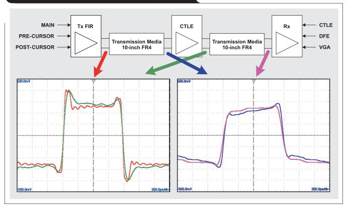
PCIe 3.0 Tx preset values at the AIC connector. PCIe 3.0 performance of the DS80PCI810 from Texas Instruments has been verified at a recent PCI-SIG Compliance Workshop. As of this article's publication, it is the only linear equalizer currently listed on the PCIe 3.0 Integrator's List. PCIe Tx presets are tested using a specific compliance pattern and oscilloscope software to extract and calculate the measurement values. This testing helps to ensure robust operation in PCIe-compliant channels.
