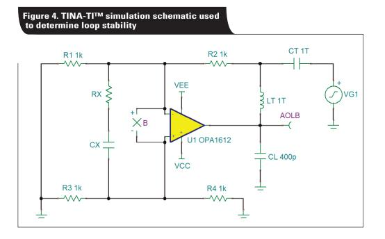
A value of 1.2 nF is very close to the calculated value for  $C_X$ . The resulting zero frequency is:
