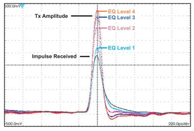
eliminating the interaction between bits, inter-symbol interference (ISI) is minimized and the eye opening is improved. This can be seen in Figure 2 by comparing the eye diagrams.
