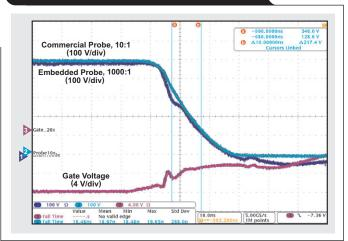
After compensation, the waveform from the embedded probe on the drain was used to estimate switching losses. Figure 7 shows how the turn-on and turn-off losses can be calculated. The total loss per cycle is the area under both triangular VI curves. To reduce measurement error, it is important to have good voltage accuracy as well as good current accuracy and skew matching (<2 ns) between both the voltage and current waveforms.
