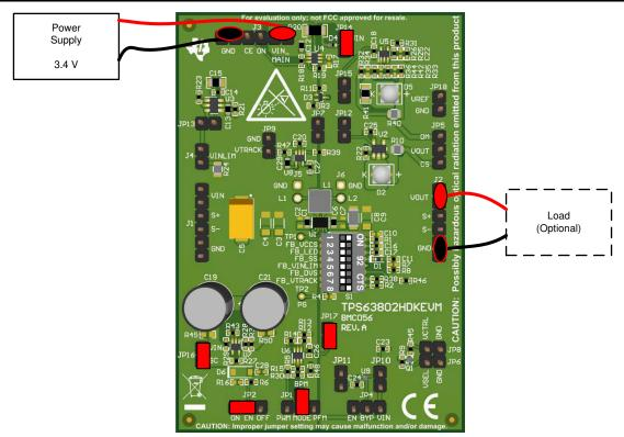
Figure 4-3. Quick Start Connection for Backup Power
