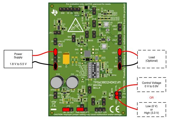
Figure 4-20. Quick Start Connection for Dynamic Voltage Scaling
