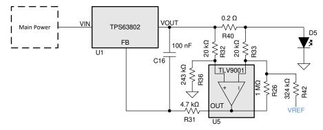
Figure 4-9. Block Diagram for High-side LED Driver with Dimming
