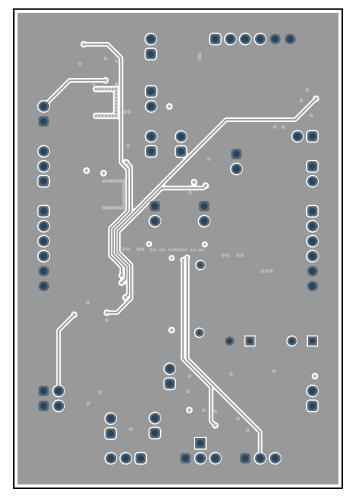
Figure 5-4. Bottom Layer Routing (Mirrored)
