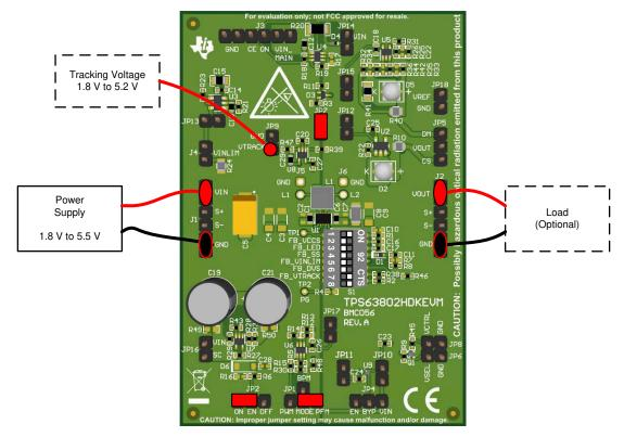
Figure 4-24. Quick Start Connection for Output Voltage Tracking
