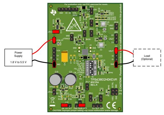
Figure 4-13. Quick Start Connection for Input Current Limitation
