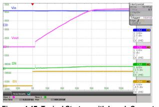
Figure 4-16. Typical Start-up Standard Operation
