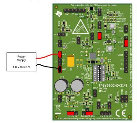
Figure 4-8. Quick Start Connection for High-side LED Driver -- Constant Current
