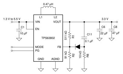
Figure 4-14. Block Diagram for Inrush Current Limitation
