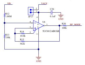
Figure 4-6. Supercapacitor Voltage Monitor
