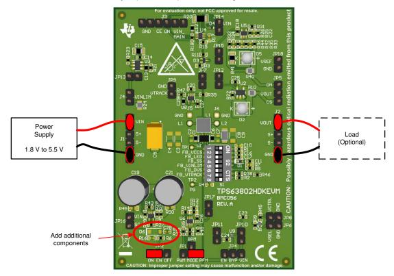
Figure 4-32. Quick Start Connection for Precise Start-up Delay
