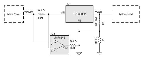
Figure 4-12. Block Diagram for Input Current Limitation
