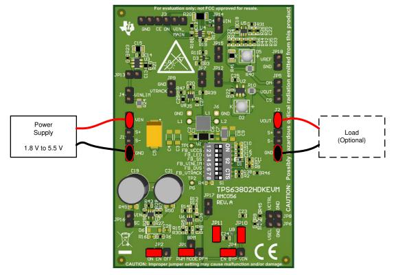
Figure 4-27. Quick Start Connection for Bypass Mode
