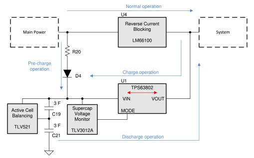
Figure 4-2. Block Diagram for Backup Power
