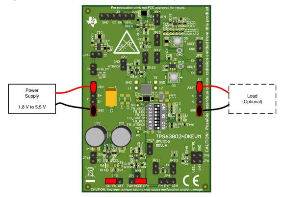
Figure 4-1. Quick Start Connection for Standard Operation
