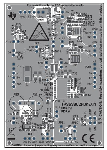
Figure 5-1. Assembly Layer
