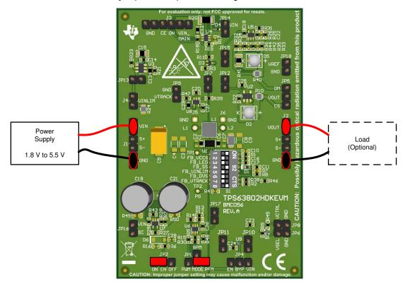
Figure 4-15. Quick Start Connection for Extending Soft Start or Inrush Rurrent Limitation
