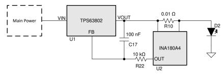
Figure 4-7. Block Diagram for High-side LED Driver -- Constant Current
