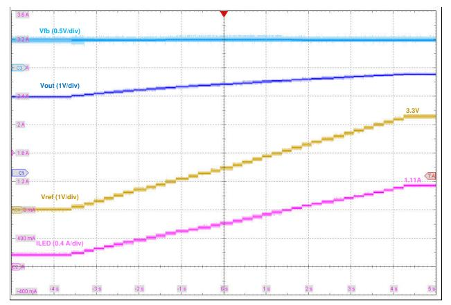
Figure 4-11. Typical Waveform Showing the LED Current in Respect to VREF
