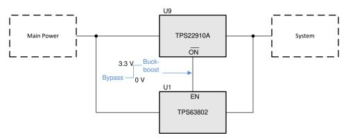
Figure 4-26. Block Diagram for Bypass Mode
