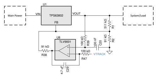
Figure 4-23. Block Diagram for Output Voltage Tracking
